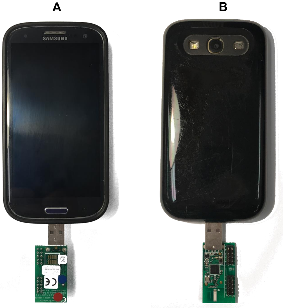
Figure S11. Mobile phone and 900 MHz wireless receiver dongle used for visualizing IMBED measurement results and logging them to the cloud. The receiver dongle connects to the phone via USB and delivers packets received wirelessly from the IMBED device to application software. The software uploads data to a cloud service and performs visualization for the user.
