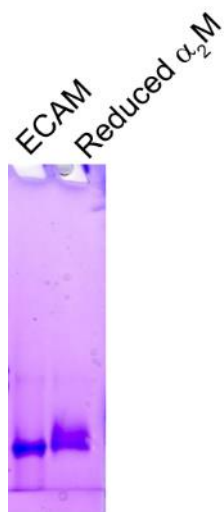
Fig. S2. Native gel image of recombinant ECAM. Image of an Instant Blue stained 3-8% Tris acetate native gel showing the migration of recombinant purified ECAM and reduced \alpha_2M .
