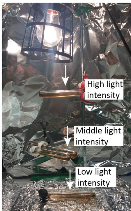
**Figure S5.** Photograph of an experiment to determine how light intensity influences the oxidation of Fe(II)-PPHA complexes by *R. ferrooxidans* SW2.
