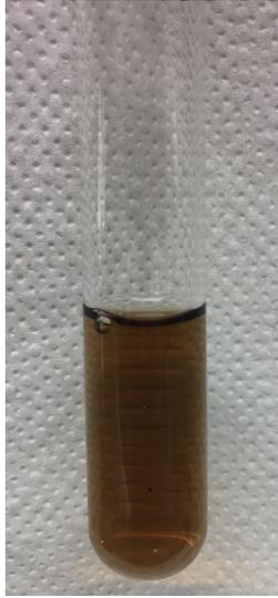
**Figure S4.** Fe(II)-PPHA complexes (0.1 mM Fe(II) and 0.2 mg/ml PPHA) in Hungate tubes. The PPHA has a dark color and absorbs light thus lowering the light intensity available for the phototrophic microorganisms.
