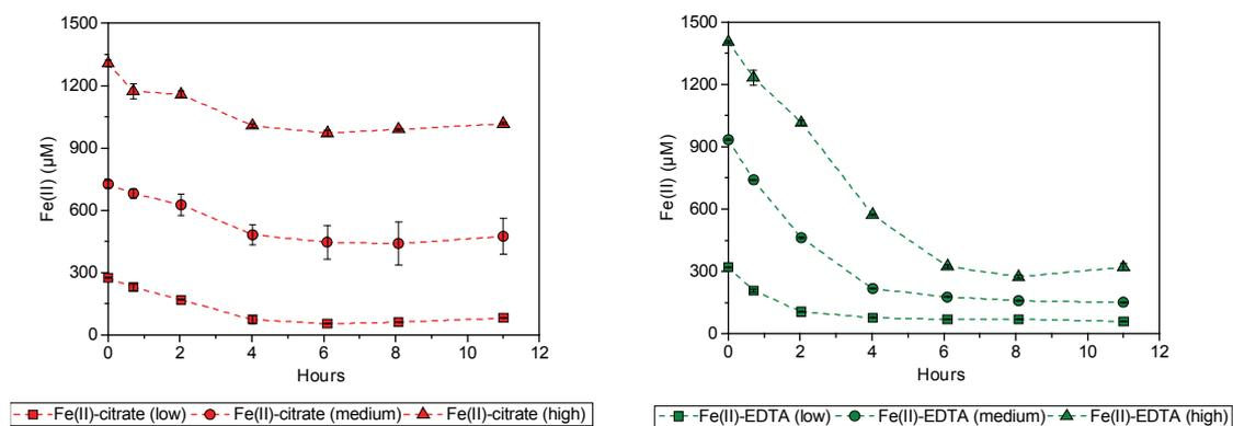
**Figure S3.** Oxidation of Fe(II)-citrate (left) and Fe(II)-EDTA (right) at three different Fe(II)-complex concentrations by *R. ferrooxidans* SW2 ( $1.4 \times 10^8$  cells/ml). The initial Fe(II) concentrations varied from ca. 300  $\mu\text{M}$  to 1300  $\mu\text{M}$ . The results are reported as an average and error bars indicate standard errors calculated from two independent parallels.
