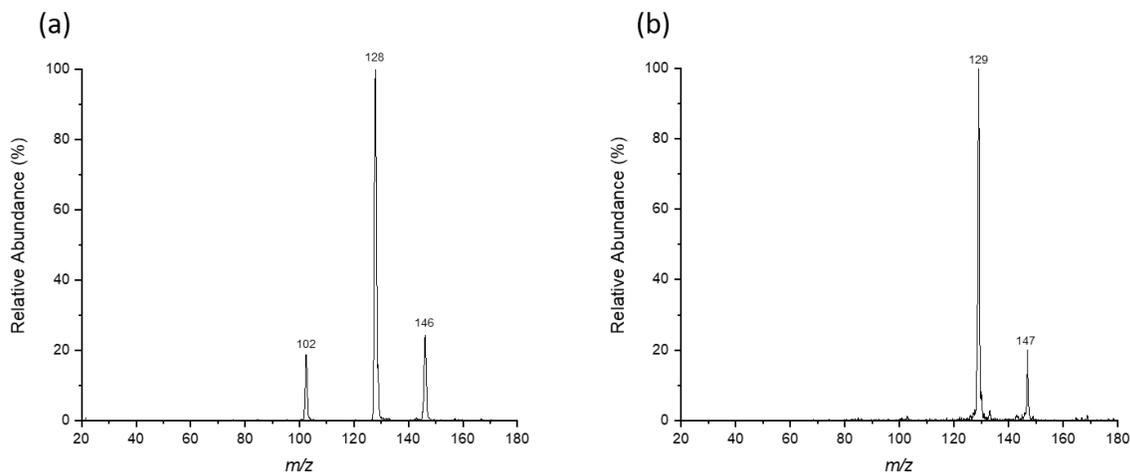
**Fig. S1** MS/MS product ion spectra recorded using Mini MS (a) GLU; (b) 2-HG
