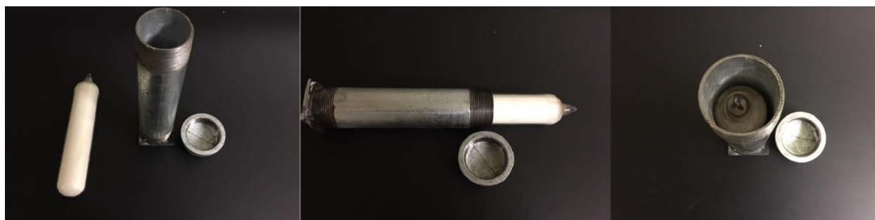
Figure S1: Example of preparing the ampule to put in the oven
