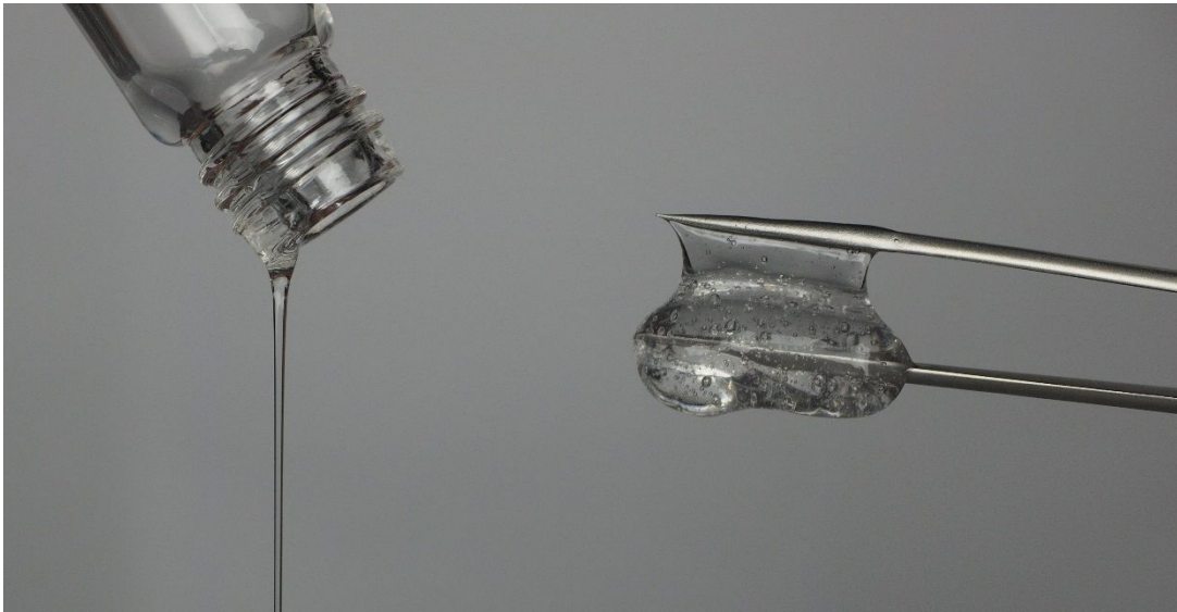
Fig.S1: Picture of the solution and putty states at a hyaluronic acid concentration of 10 mg/ml.
