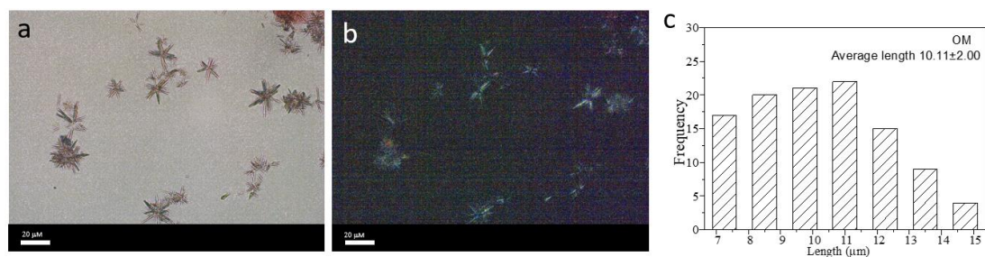
Figure S26. Optical (a) and polarized (b) images of needle-based flowers contained lysine-modified perylene. (c) Corresponding histogram.
