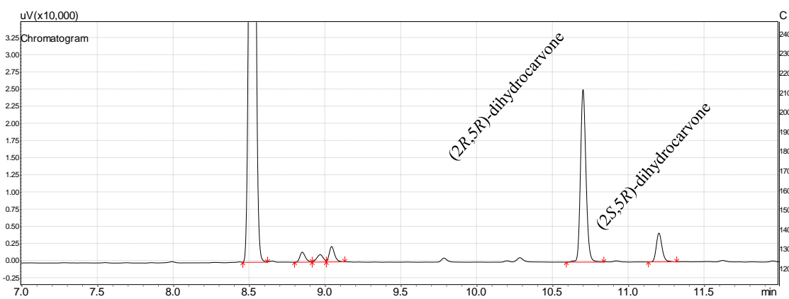
Representative GC chromatogram showing the baseline separation of (2R,5R)- and (2S,5R)-dihydrocarvone.
