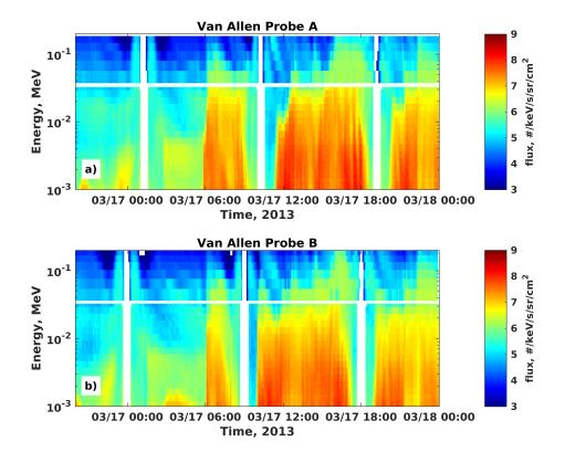
Figure 1. Combined HOPE and MagEIS spectrum for 90° local pitch angle for the Van Allen Probes A (a) and B (b). The HOPE data above 30 keV are not shown, and the white horizontal line marks the energy boundary between the instruments.
