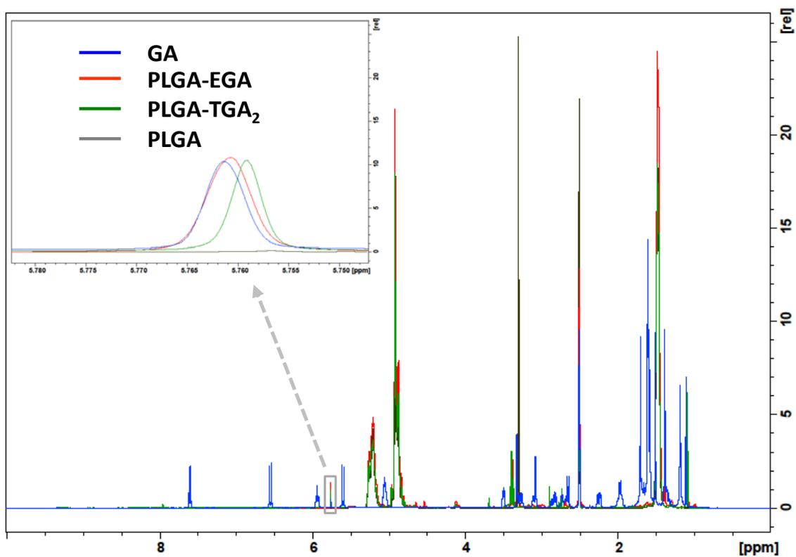
Fig. S10.  $^1\text{H}$  NMR of GA, PLGA-EGA, PLGA-TGA<sub>2</sub> and PLGA with the inset highlighting GA representative peaks.
