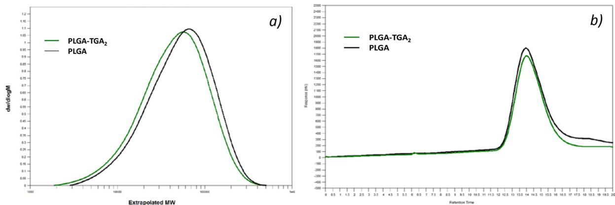
Fig. S11. a) Molecular weight and b) distribution profiles of PLGA and PLGA-TGA<sub>2</sub> obtained from GPC
