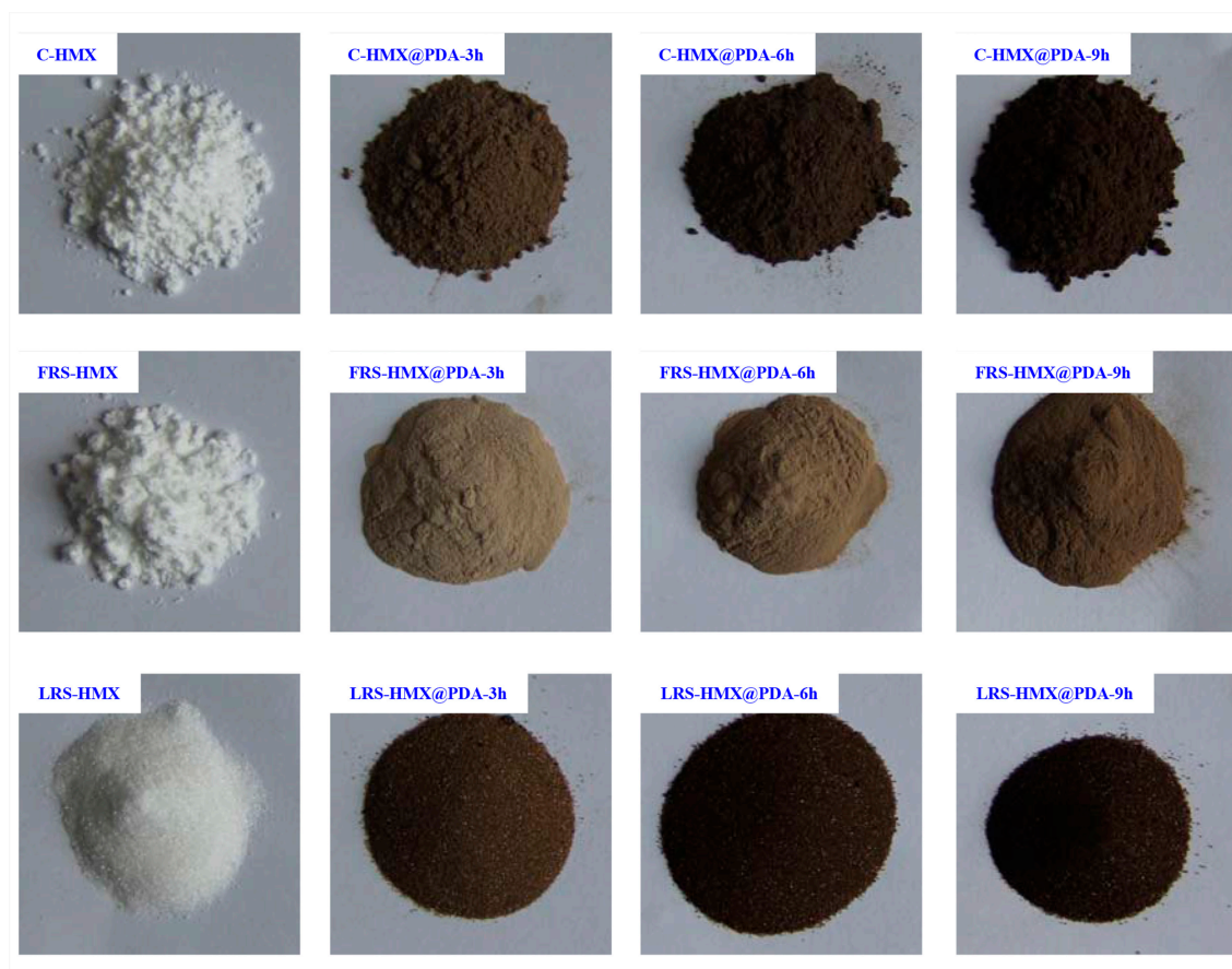
Fig. S2. Photos of HMX crystals and HMX@PDA composites.
