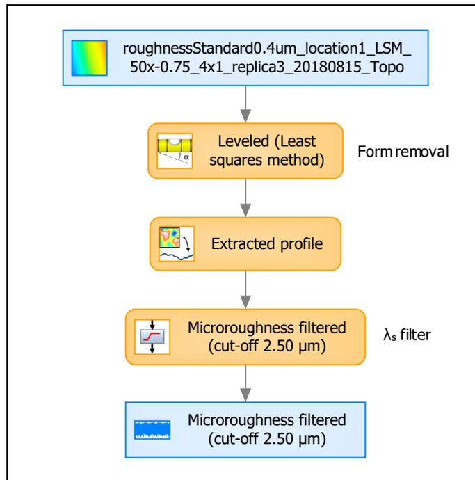
**Roughness standard  $Ra = 0.4 \mu\text{m}$
