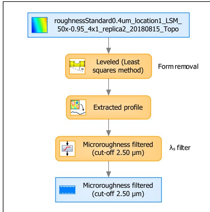
**Roughness standard  $Ra = 0.4 \mu\text{m}$
