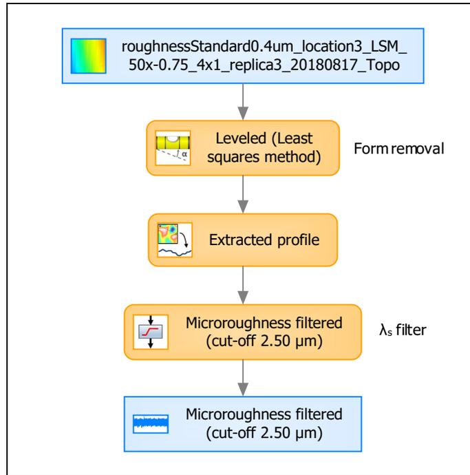
**Roughness standard  $Ra = 0.4 \mu\text{m}$
