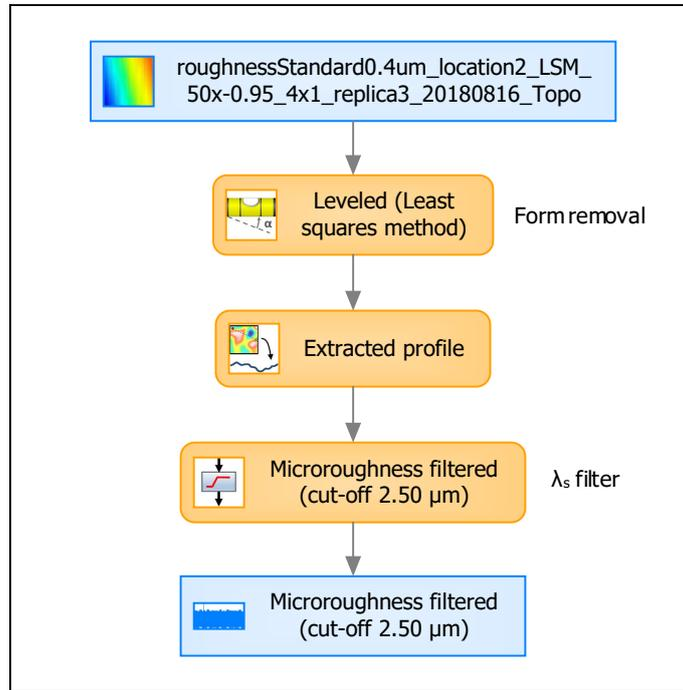
**Roughness standard  $Ra = 0.4 \mu\text{m}$
