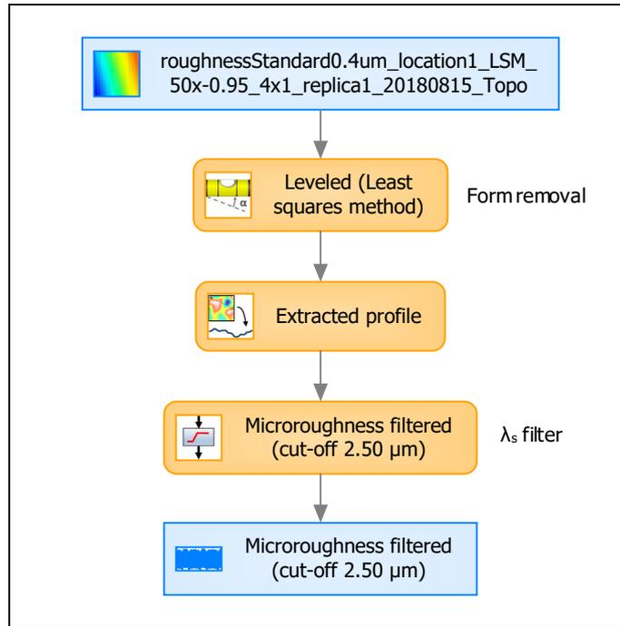
**Roughness standard  $Ra = 0.4 \mu\text{m}$
