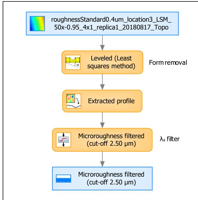
**Roughness standard  $Ra = 0.4 \mu\text{m}$
