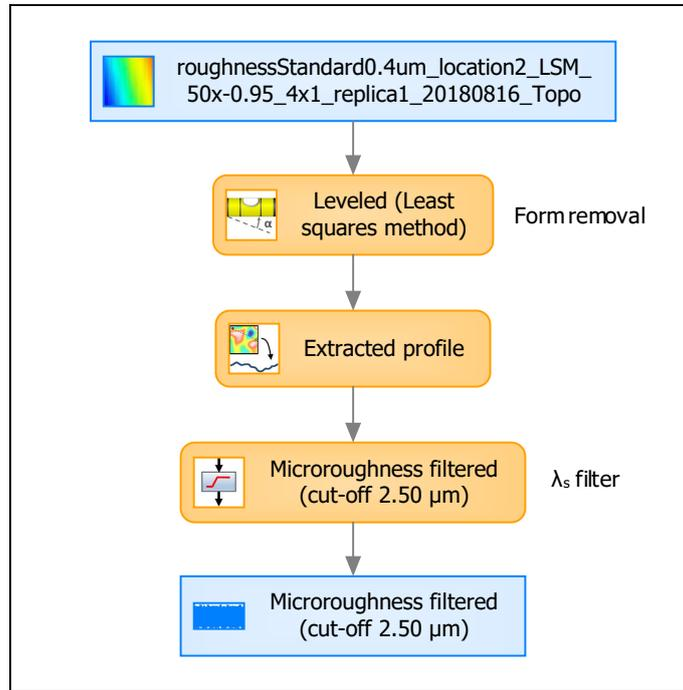
**Roughness standard  $Ra = 0.4 \mu\text{m}$
