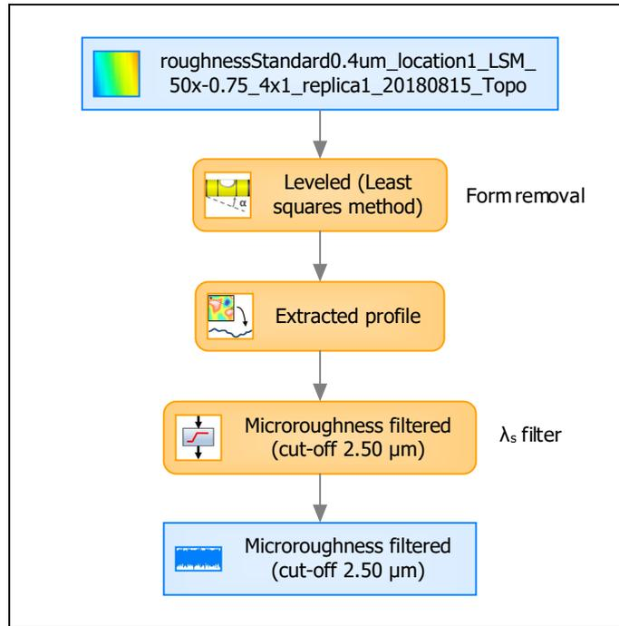
**Roughness standard  $Ra = 0.4 \mu\text{m}$
