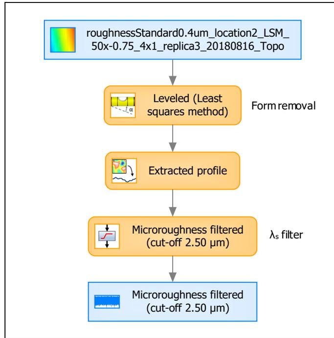
**Roughness standard  $Ra = 0.4 \mu\text{m}$
