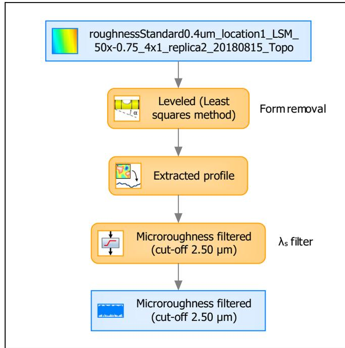
**Roughness standard  $Ra = 0.4 \mu\text{m}$
