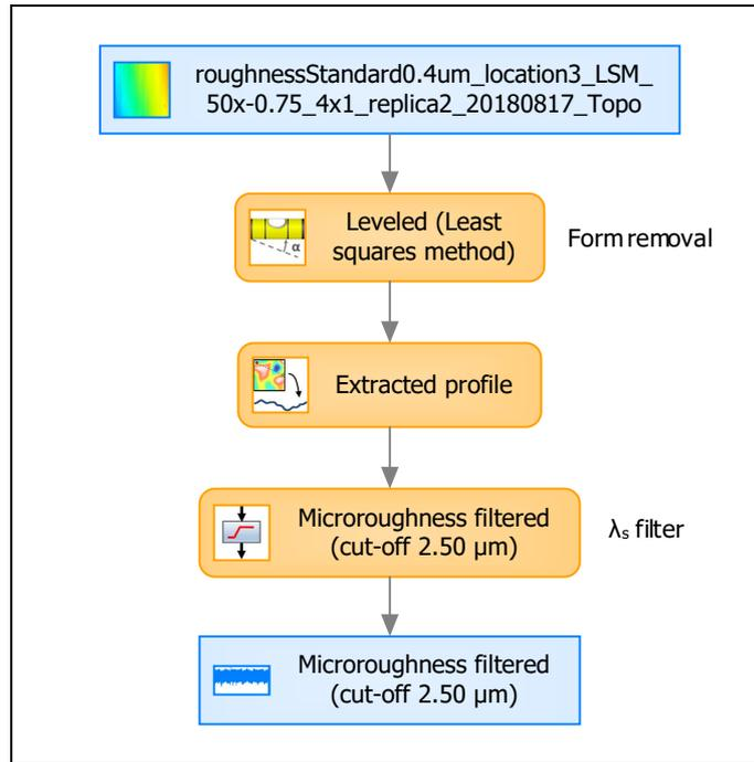
**Roughness standard  $Ra = 0.4 \mu\text{m}$
