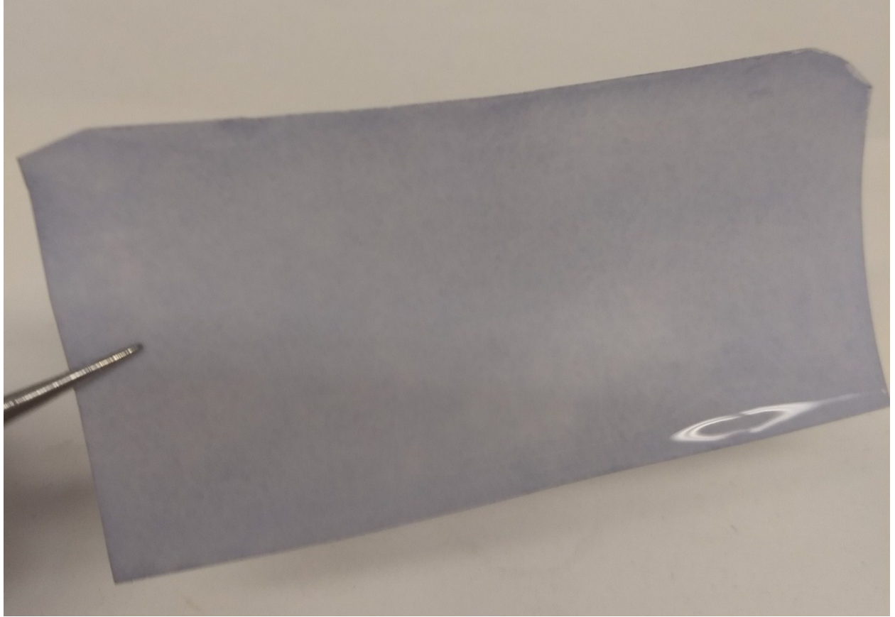
Figure S3. Photo showing a modified PES membrane which has been kept in water for almost one year.
