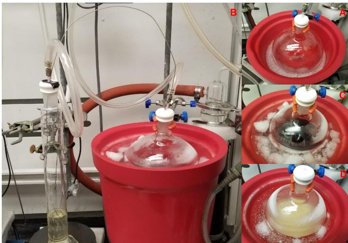
**Picture S4. Synthesis of lactam 35.** (A) Initial solution of (+)-epoxyacetone **14** in THF. (B) Cannulation of *t*BuLi into the reaction vessel. (C) Reaction mixture after addition of *t*BuLi. (D) Reaction mixture after addition of sat. aq. NH<sub>4</sub>Cl.
