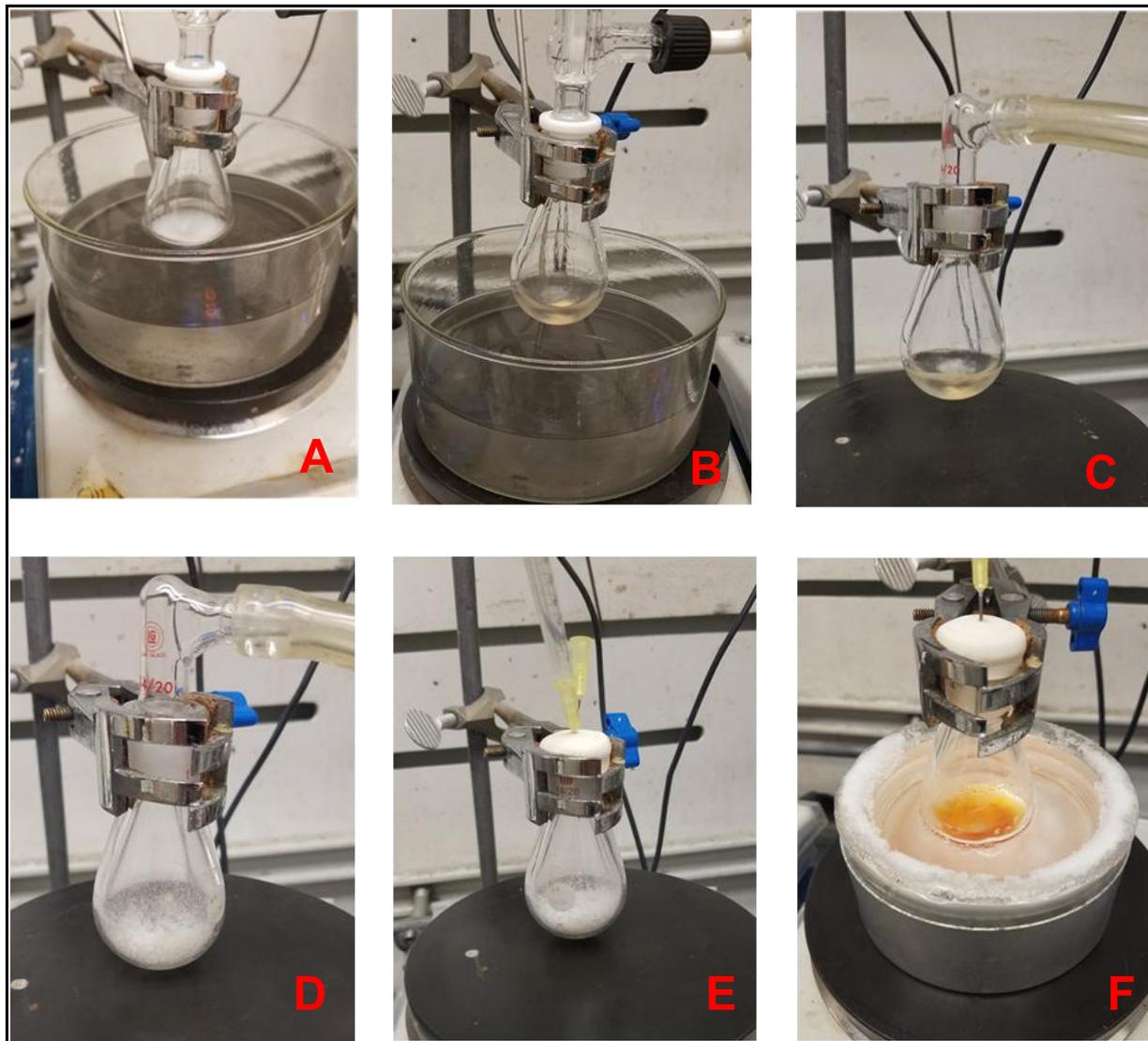
**Picture S3. Synthesis of pancratistatin.** (A) Initial suspension of (+)-7-deoxypancratistatin (**1**) in HMDS/MeCN. (B) Reaction mixture after 12 h at 80 °C. (C) Removal of volatiles under reduced pressure. (D) Leftover residue after azeotropic co-evaporation. (E) Nitrogen purge. (F) Reaction mixture after addition of  $(\text{TMP})_2\text{Cu}(\text{CN})\text{Li}_2$ .
