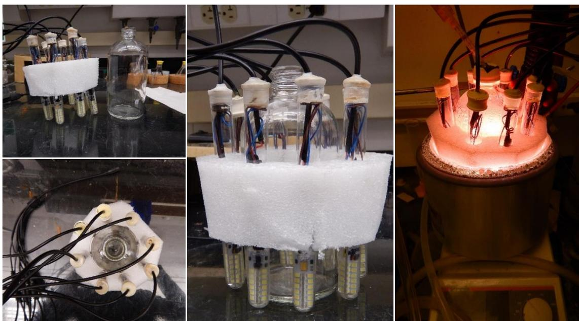
Picture S1. Photochemical set-up for dearomative *trans*-1,2-carboamination.
