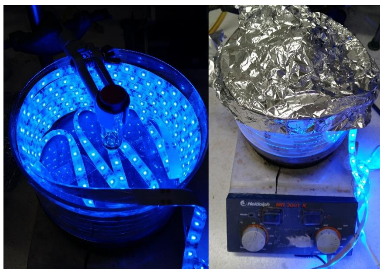
Figure S1a: Reaction setup for secondary/benzylic alkylpyridinium salts (GP2, GP4)
