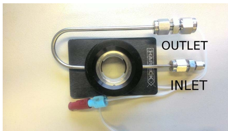
Figure 2: IR chamber for in-situ acquisition. The inlet and outlet are highlighted.
