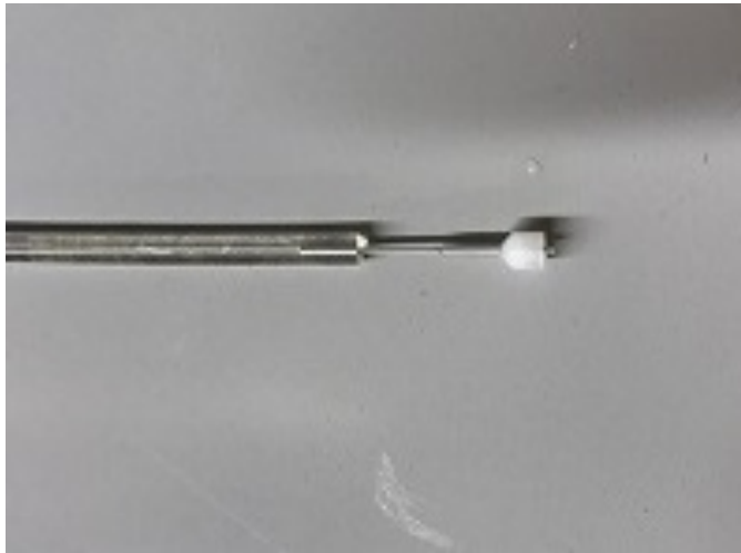
Supplementary Figure 1. Supradural injectors, tubing, and Hamilton syringe. (Left) Mouse dural injectors were modified from commercially available internal cannulas (Invivo1, part #C313I/SPC). The injector projection length (0.5mm to 0.65mm) varied depending upon the weight of each mouse. (Right) The modified injectors were attached to a 10 \mu l glass syringe cemented needle (Hamilton Company, 700 series) via tygon tubing (Cole-Palmer, Item # EW-96460-16).
