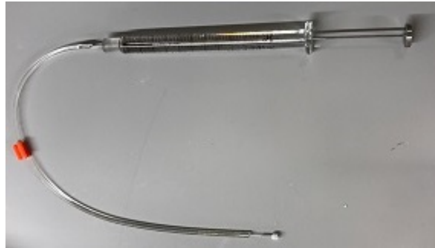
Supplementary Figure 1. Supradural injectors, tubing, and Hamilton syringe. (Left) Mouse dural injectors were modified from commercially available internal cannulas (Invivo1, part #C313I/SPC). The injector projection length (0.5mm to 0.65mm) varied depending upon the weight of each mouse. (Right) The modified injectors were attached to a 10 \mu l glass syringe cemented needle (Hamilton Company, 700 series) via tygon tubing (Cole-Palmer, Item # EW-96460-16).
