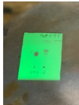
Left: Reaction after 10 mins. Center: Reaction after 20 hours. Right: TLC for starting material (left) and crude reaction mixture (right, top spot is the product).
