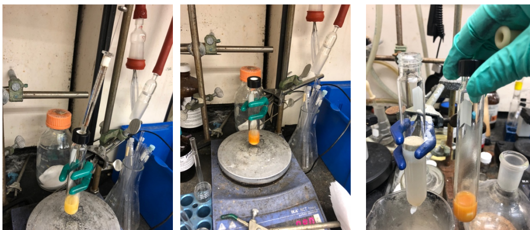
Left: Adding DIC. Center: stir at room temperature for 2 hours. Right: Column chromatography for purification.
