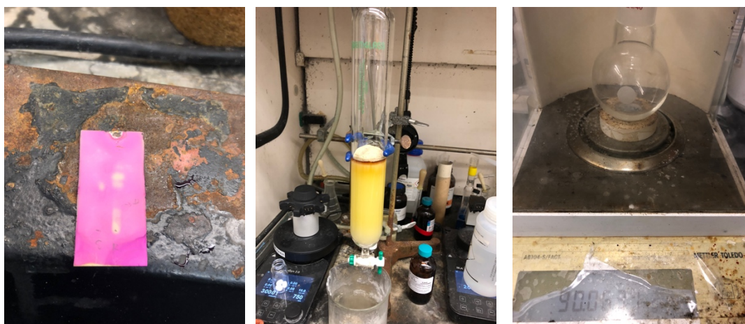
Left: TLC for starting material (left) and crude reaction mixture (right, top spot is the product). Center: Column chromatography. Right: Weight of the empty flask for product.
