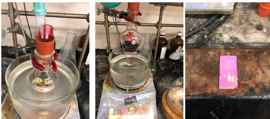
Left: Bubbling during the reaction. Center: Reaction completed after 6 hours. Right: TLC for starting material (left) and crude reaction mixture (right two, bottom spot is the product).
