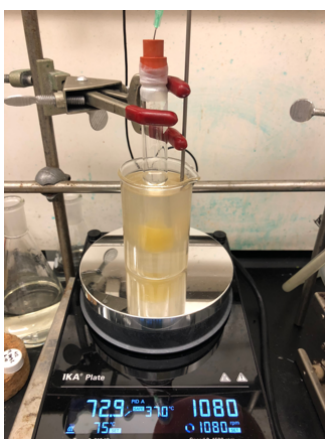
Addition of catalyst stock solution. Center: The culture tube placed at 75 °C. Right: The reaction mixture after 12 hours.
