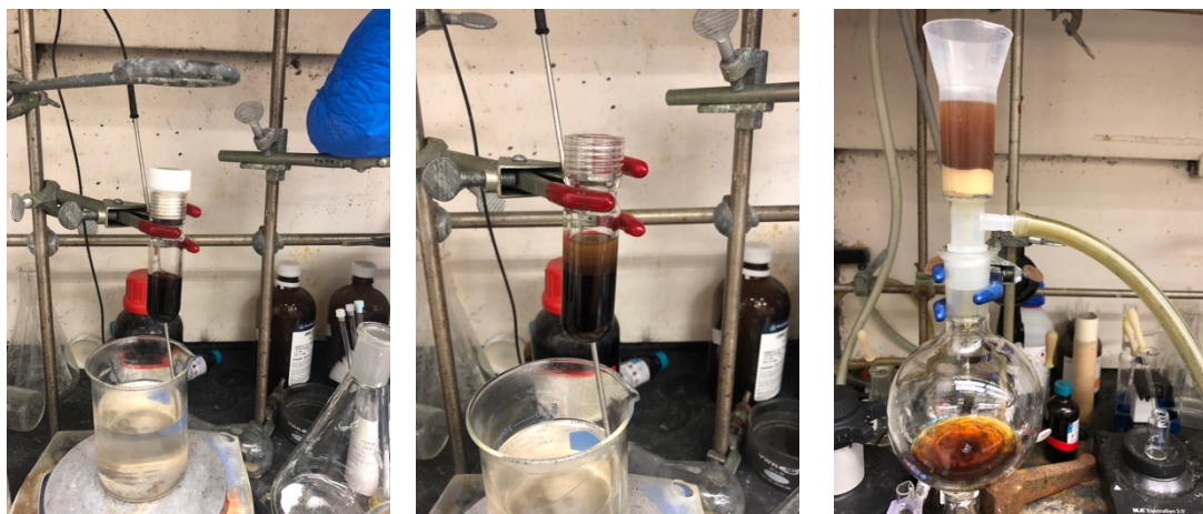
Left: Reaction after 12 hours. Center: Dilute the reaction with EtOAc (5 mL). Right: Filter through a pad of Celite®.
