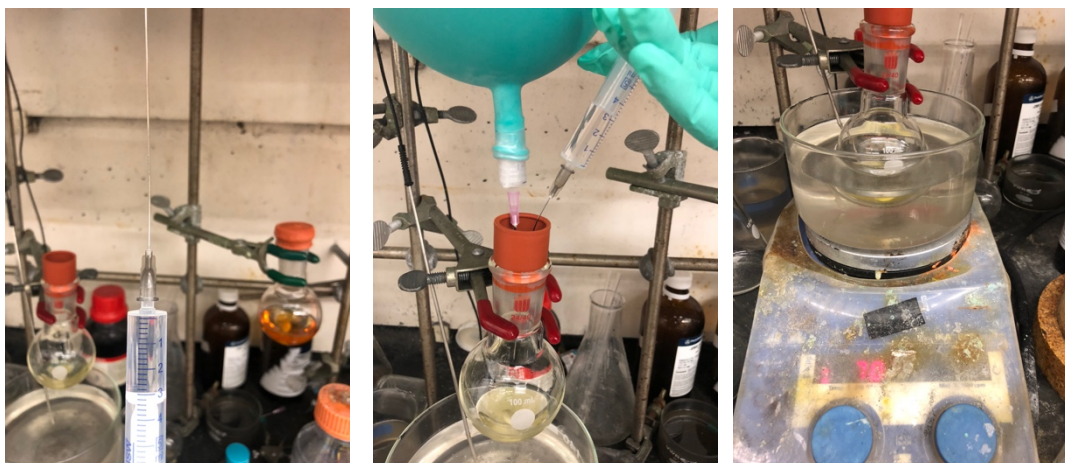
Left: \text{Boc}_2\text{O} . Center: Adding \text{Boc}_2\text{O} slowly. Right: Put the flask into a preheated oil bath (70 °C).
