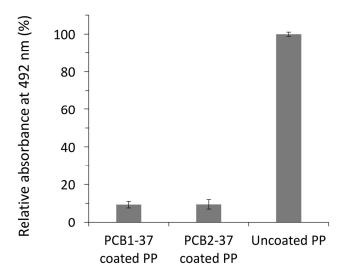
**Figure S-2.** Relative adsorption of fibrinogen (1.0 mg/mL,  $1 \times$  PBS, pH 7.4) on PP surfaces coated with (a) PCB1-37 and (b) PCB2-37 at 0.5 wt% concentration.
