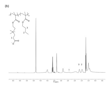
**Figure S-1.** <sup>1</sup>H-NMR spectrum of (a) poly(CB1-*co*-BMA) (PCB1); and (b) poly(CB2-*co*-BMA) (PCB2). CB1: 1-Carboxy-*N*,*N*-dimethyl-*N*-(3'-acrylamidopropyl) ethanaminium inner salt; CB2: carboxybetaine methacrylate, 2-carboxy-*N*,*N*-dimethyl-*N*-(2'-methacryloyloxyethyl) ethanaminium inner salt; BMA: *n*-butyl methacrylate.
