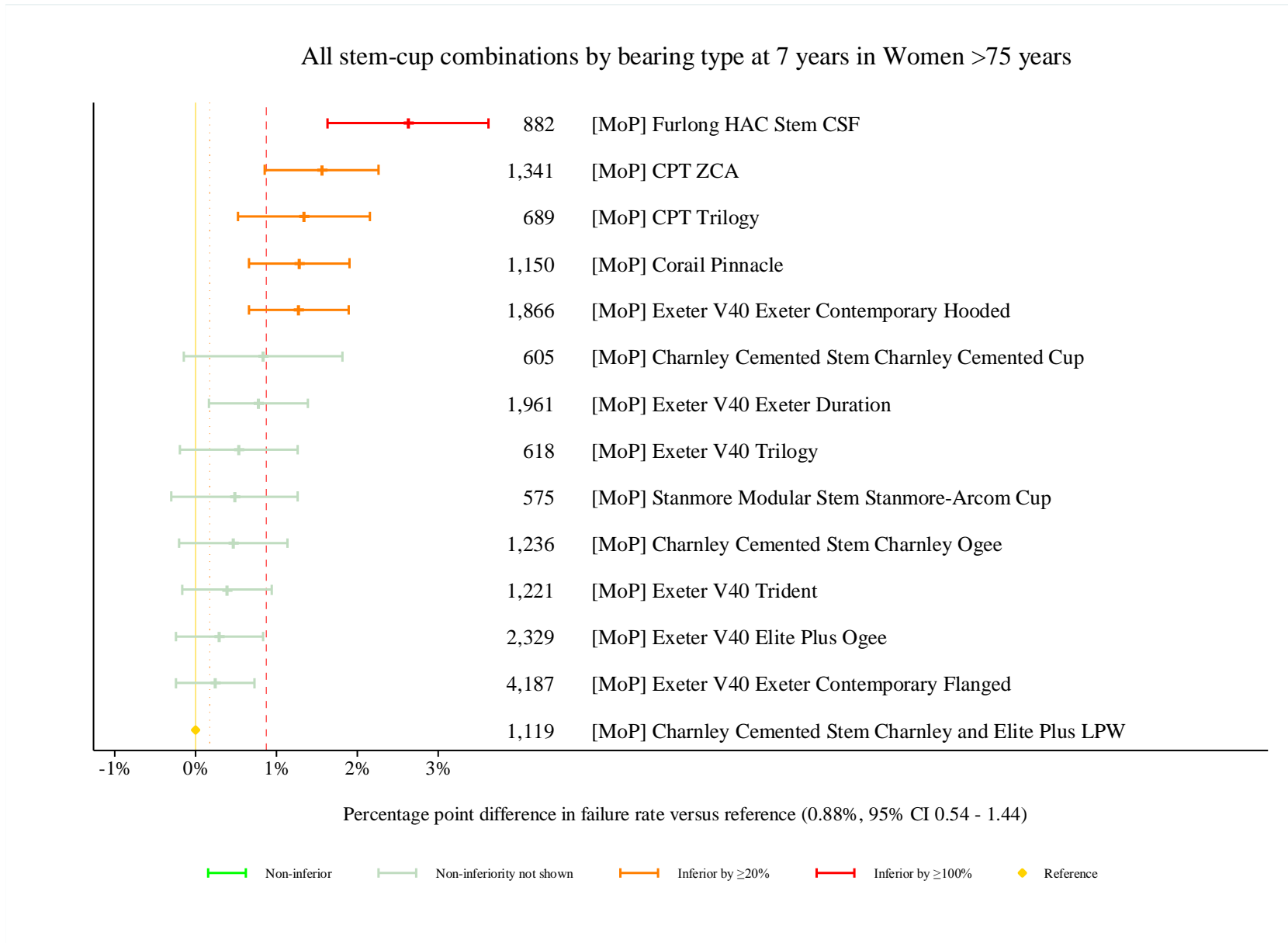
Supplementary Figure 8d: Difference in failure of implanted constructs compared to a contemporary reference at 7 years in women greater than 75 years, using all stem-cup combinations with \geq 500 procedures remaining at risk
