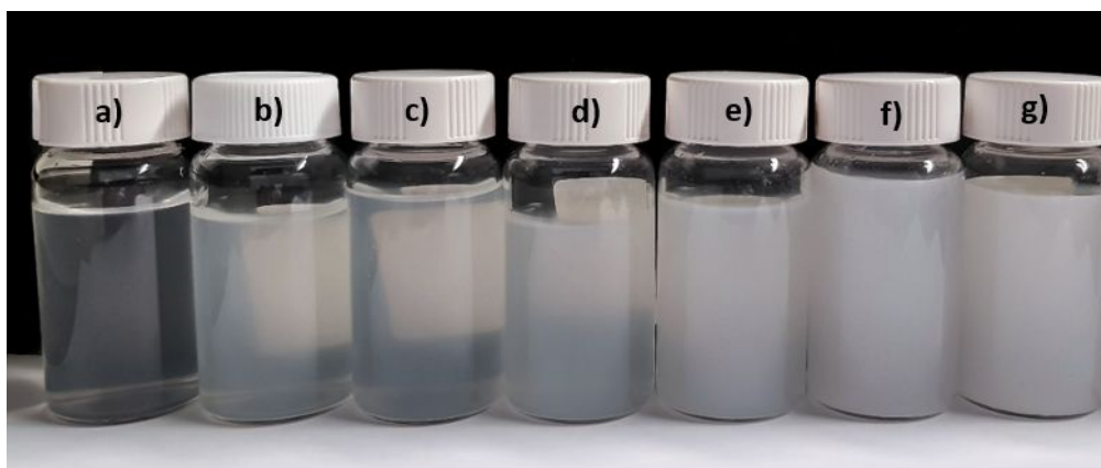
Figure S1. Photographs of CNF-stabilized Pickering emulsions with different oil concentrations a) Reference (CNF, 0.05wt%); b) 0.01wt% oil; c) 0.016 wt% oil; d) 0.025 wt% oil; e) 0.05 wt% oil; f) 0.24 wt% oil and g) 0.33 wt% oil. All emulsions contain 0.05wt% CNF.
