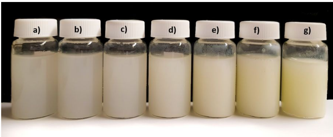
Figure S10. Photographs of CNF-stabilized Pickering emulsions with different oil concentrations loaded with curcumin ( 5.5 \times 10^{-6} wt% in oil phase): a) 0.1 wt% oil; b) 0.0166
