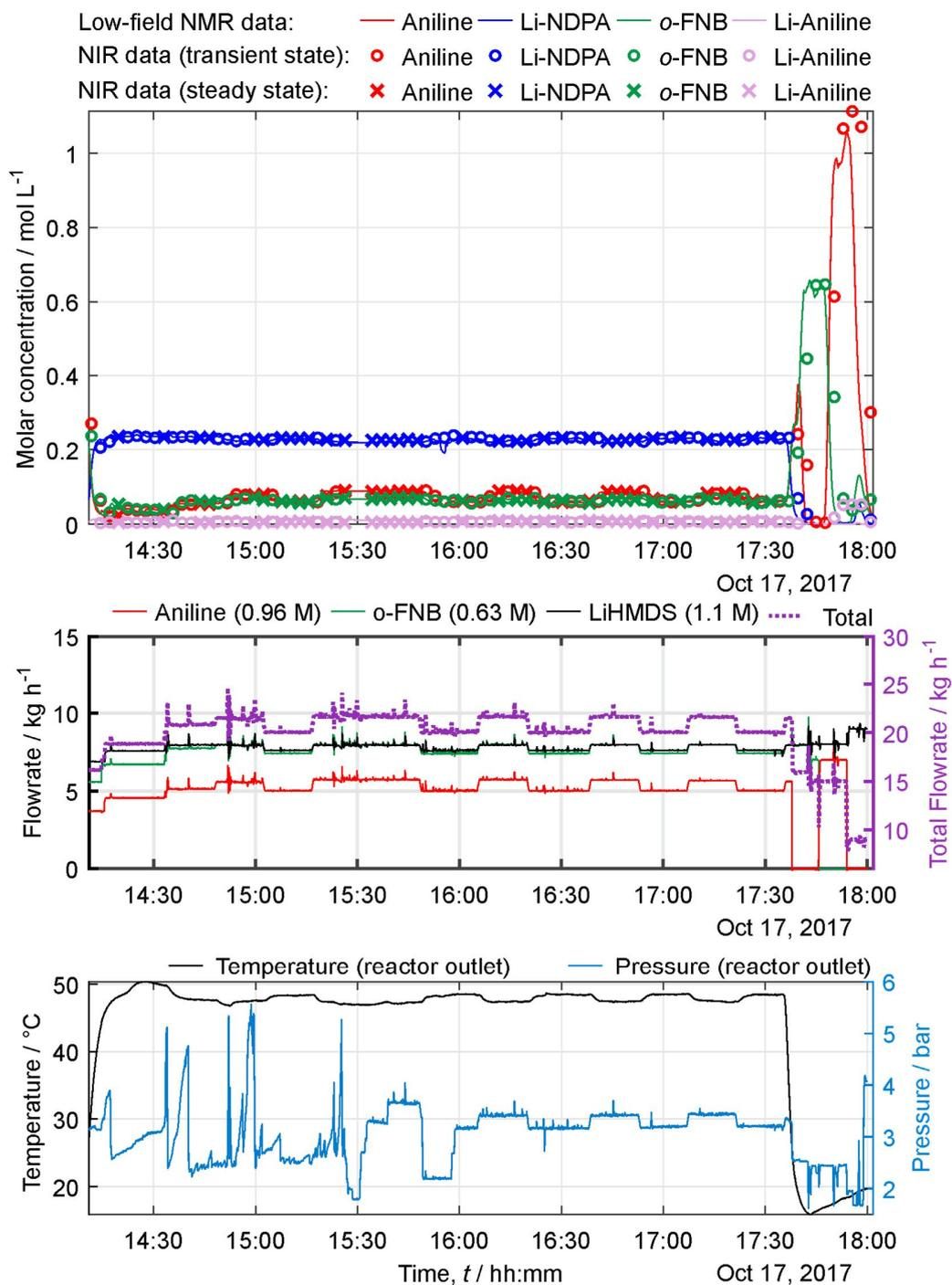
**Fig. S14** Time course of relevant process data during continuous NDPA synthesis in the modular production plant (17.10.2017, production day 4, part B)
