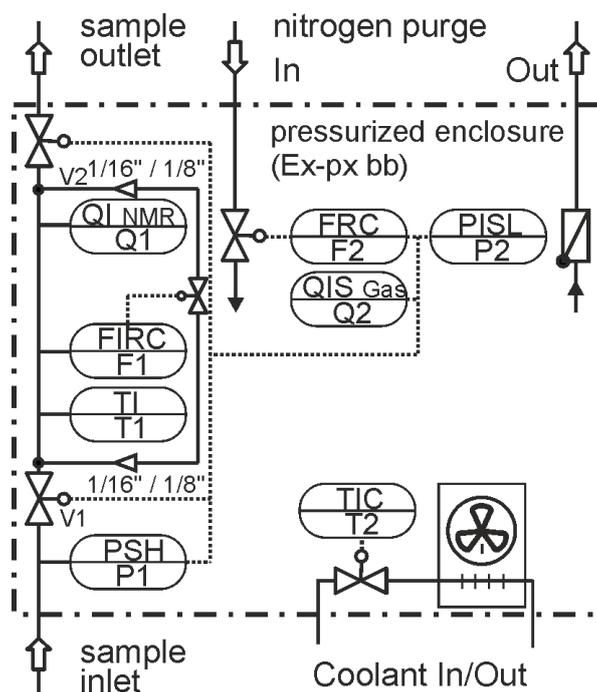
**Fig. S2** P&ID of the online NMR module. Set-up with variable sample flow ( $>10 \text{ mL min}^{-1}$ ) whereby the flow through the NMR spectrometer is kept constant at  $1.5 \text{ mL min}^{-1}$ . The thresholds leading to the closing of safety valves V1 and V2 were implemented as follows: P1, 9.3 bar; P2, 0.89 mbar; Q1: 1000 ppm (vol/vol THF)
