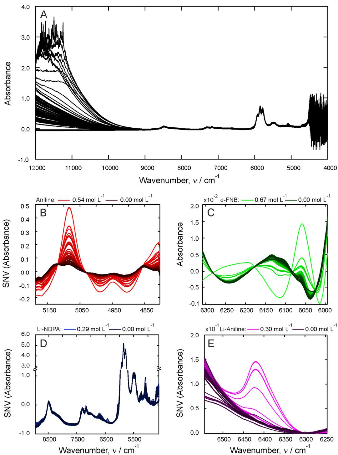
**Fig. S5** Measured NIR spectra over the full spectral range of steady states during three test runs on days one two, and four comprising the calibration set (A). B–E shows pretreated spectra according to Table S1. Based on individually optimized spectral pretreatment strategies for the reactants aniline (B), *o*-FNB (C), the product Li-NDPA (D) and lithiated aniline (E), individual PLS1 models were developed using NMR concentration values as a reference
