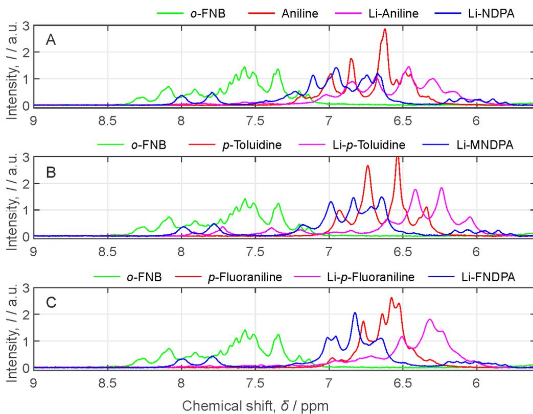
**Fig. S1** Measured pure substance spectra of the reactants dissolved in THF, which occurred during the continuous synthesis of 2-nitrodiphenylamine (A, NDPA), 2-nitro-4'-methyldiphenylamine (B, MNDPA), and 2-nitro-4'-fluorodiphenylamine (C, FNDPA).  $^1\text{H}$  spectra (43 MHz) were recorded as a single scan
