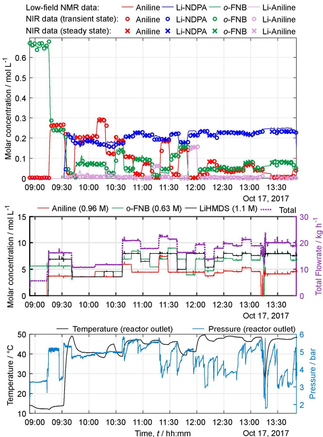
**Fig. S13** Time course of relevant process data during continuous NDPA synthesis in the modular production plant (17.10.2017, production day 4, part A). Probing moves were performed between 9:15 h and 13:30 h. Subsequently the MAWQA algorithm was initialized
