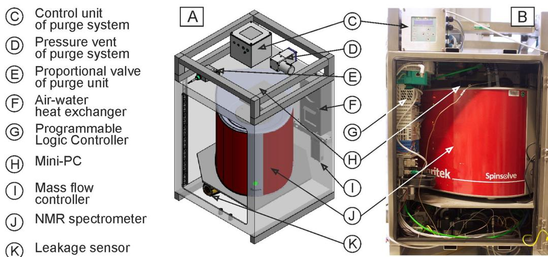
**Fig. S3** Spatial arrangement of the components of the online NMR module, including a pressurized enclosure system during the design phase (A) and after system integration (B)
