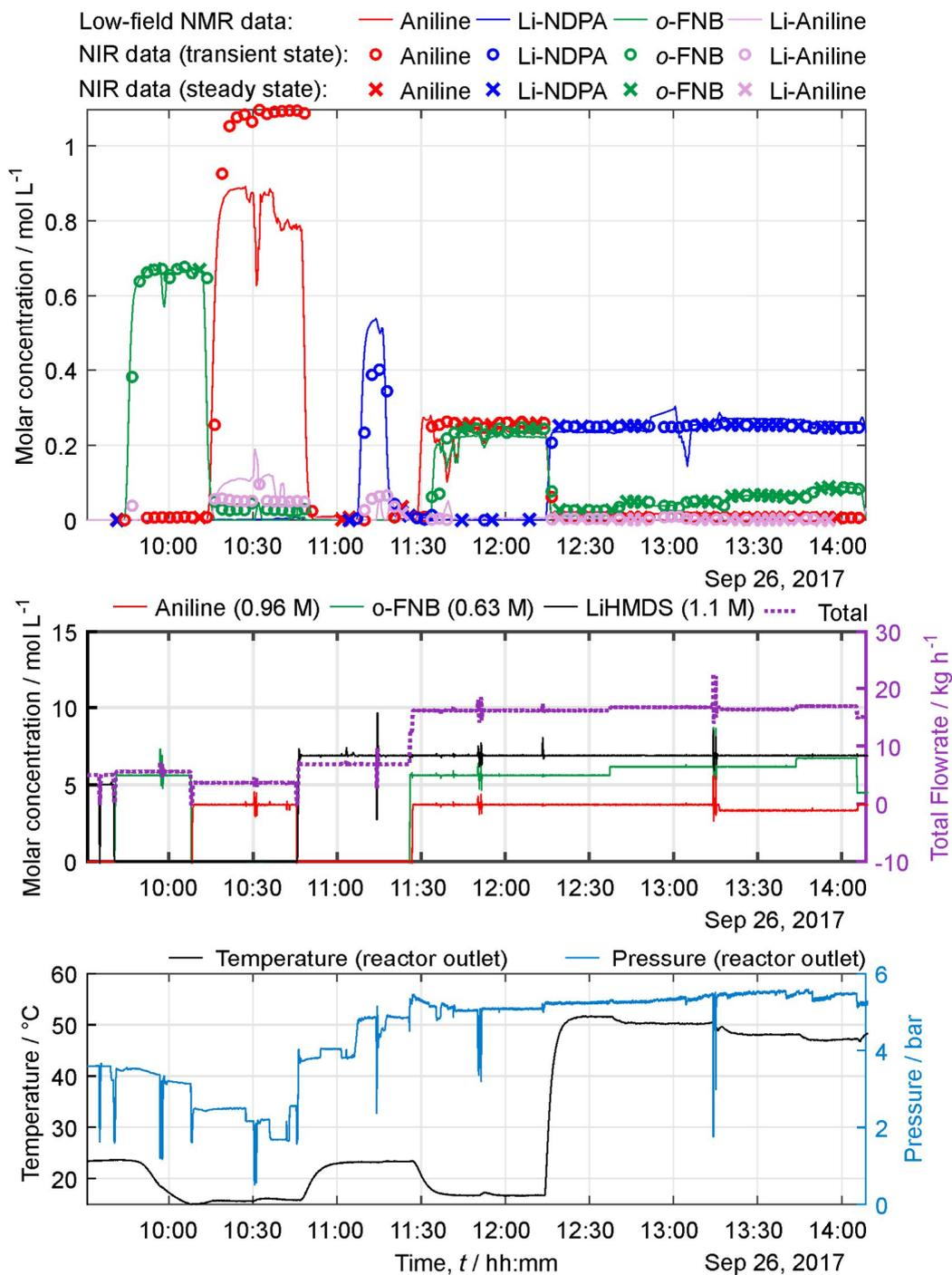
**Fig. S7** Time course of relevant process data during continuous NDPA synthesis in the modular production plant (26.09.2017, production day 1, part A)
