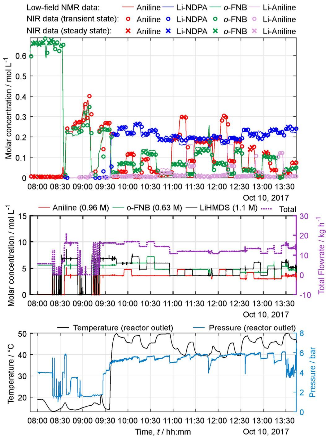
**Fig. S11** Time course of relevant process data during continuous NDPA synthesis in the modular production plant (10.10.2017, production day 3, part A)
