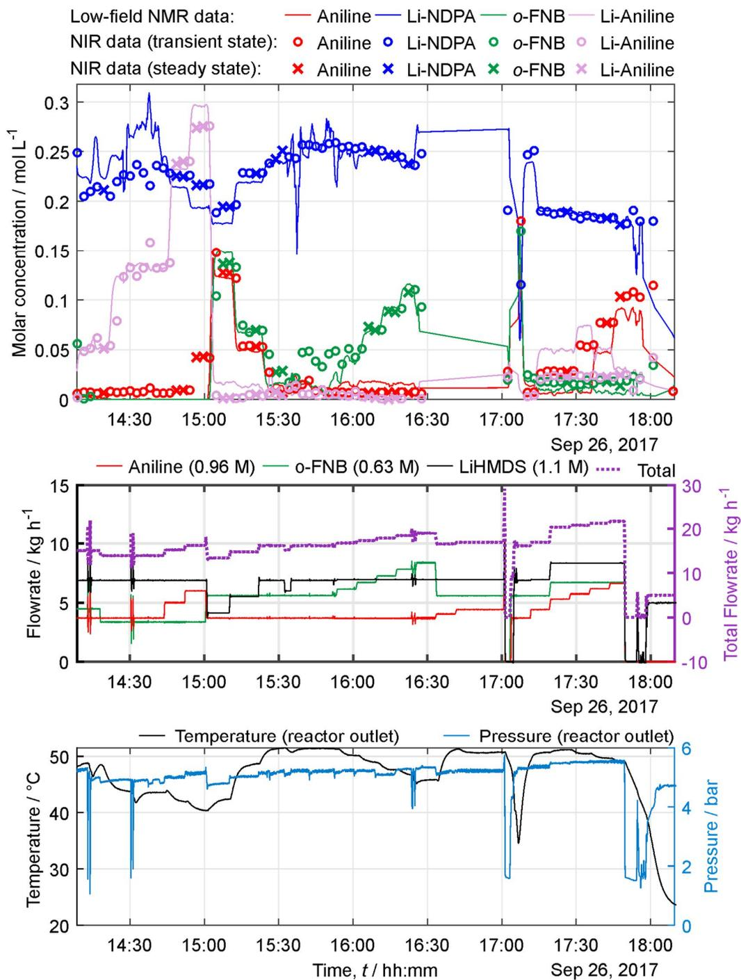
**Fig. S8** Time course of relevant process data during continuous NDPA synthesis in the modular production plant (26.09.2017, production day 1, part B)
