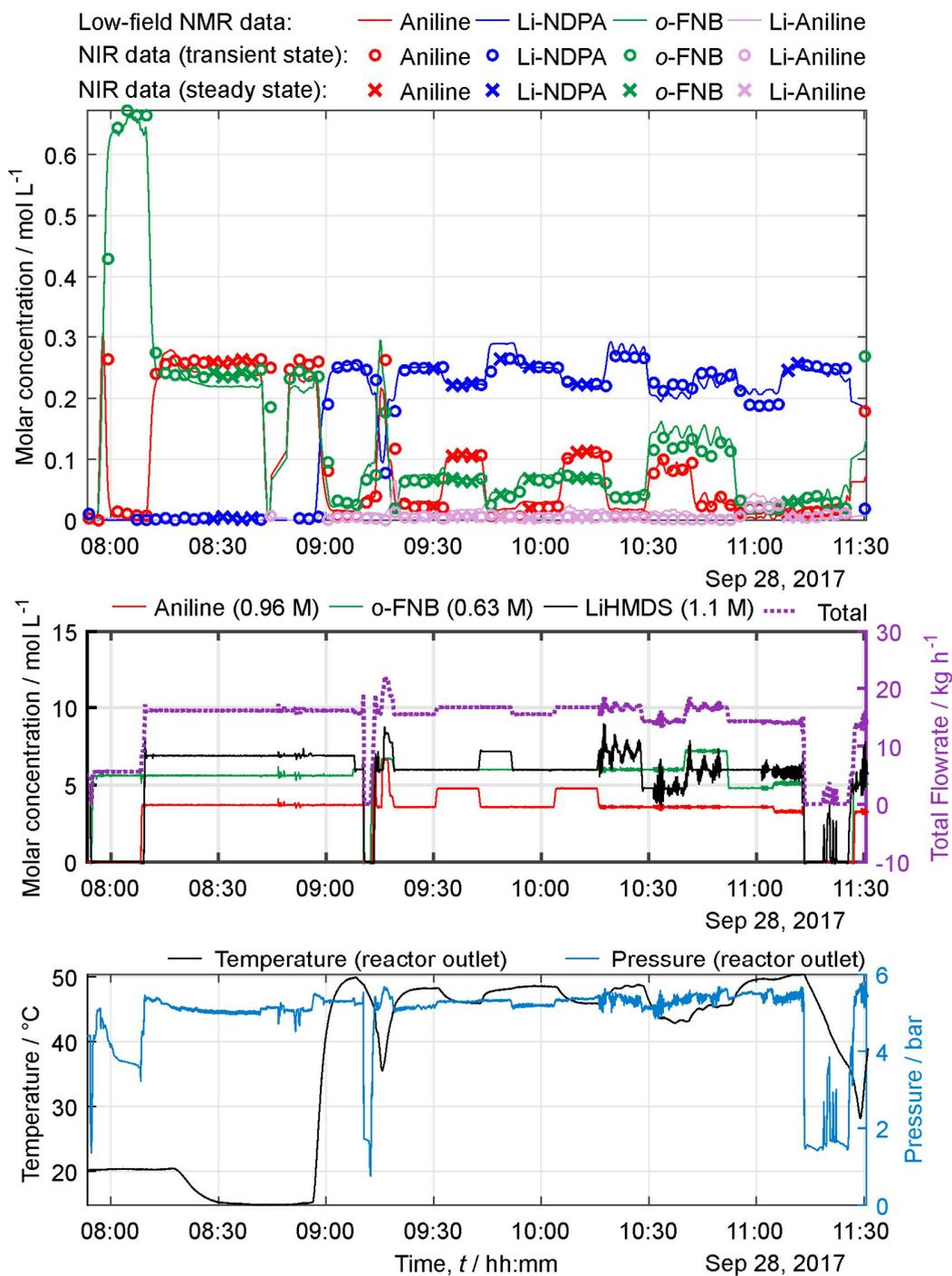
**Fig. S9** Time course of relevant process data during continuous NDPA synthesis in the modular production plant (28.09.2017, production day 2, part A)
