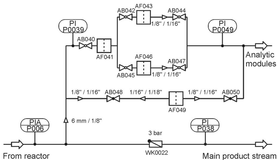
**Fig. S4** P&ID of the filter section within the bypass to the analytic modules (NMR and NIR). A combination of 90  $\mu\text{m}$  (AF041) and 60  $\mu\text{m}$  (AF043 and Af046) stainless steel inline filters (Swagelok) has evolved as a robust arrangement to prevent clogging of the bypass. Due to the redundant design of the filter section, exchange of clogged filters during the production was possible
