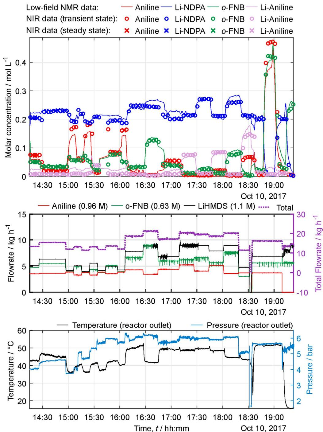
**Fig. S12** Time course of relevant process data during continuous NDPA synthesis in the modular production plant (10.10.2017, production day 3, part B)
