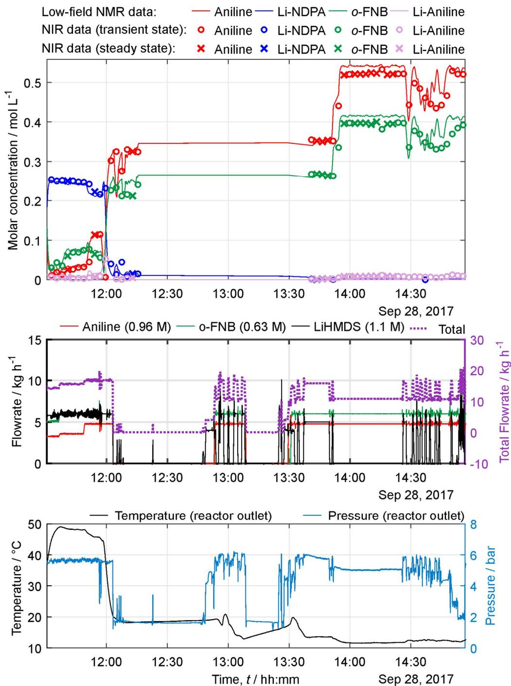
**Fig. S10** Time course of relevant process data during continuous NDPA synthesis in the modular production plant (28.09.2017, production day 2, part B)
