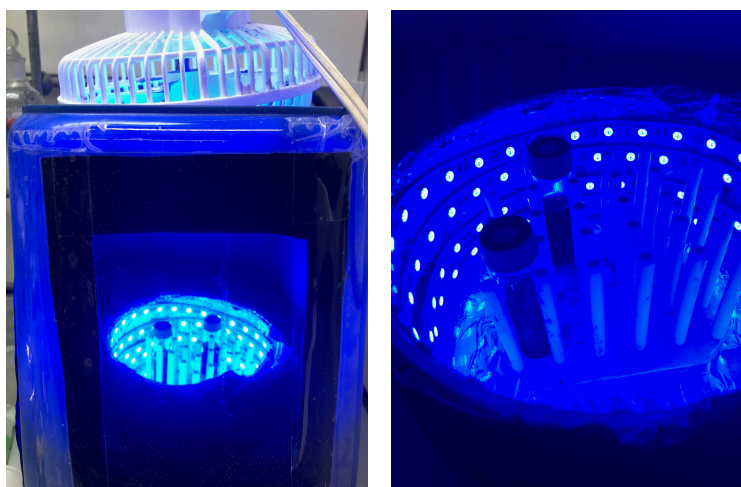
Figure 2. Reaction set up with blue LED strips. 1
