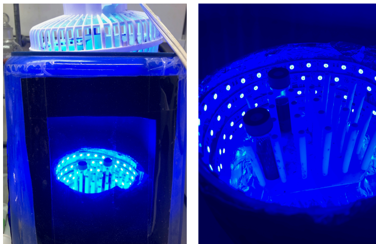
Figure 2. Reaction set up with blue LED strips. 1
