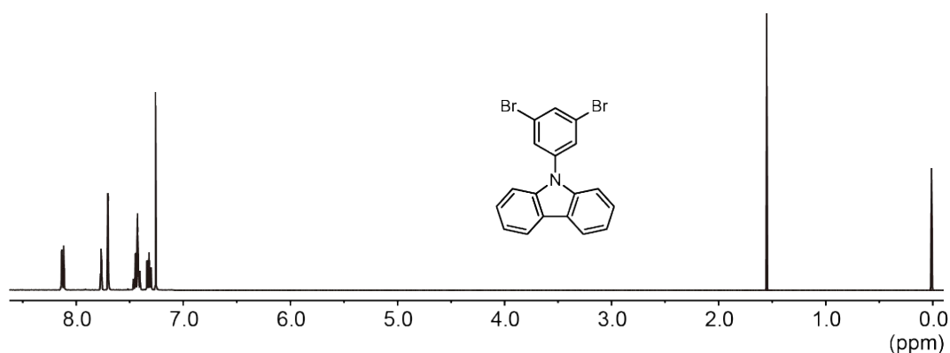
Figure S7. ^1\text{H} NMR spectrum of 9-(3,5-dibromophenyl)-9H-carbazole ( DBrPhCz ).
