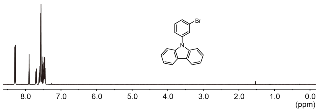
Figure S5. ^1\text{H} NMR spectrum of 9-(3-bromophenyl)-9H-carbazole ( mBrPhCz ).
