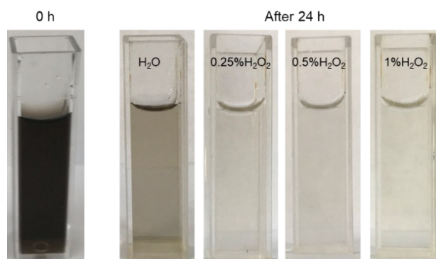
Figure S6. Digital photographs of Re nanoclusters dispersions with a concentration of 500 ppm after incubation in H 2 O, 0.25%, 0.5% and 1% H 2 O 2 solution for 24 h.
