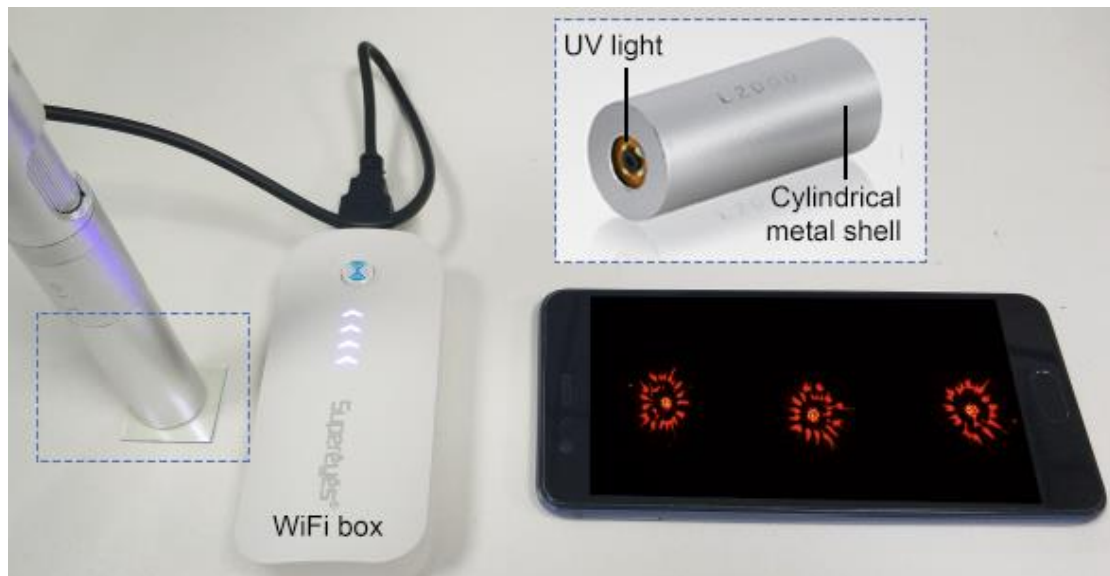
Supplementary Figure 7. Pattern readout with a smartphone microscope: the portable mini-microscope is composed of a UV chip, a 200× magnification-adjustable objective lens covered with a cylindrical metal shell and a small WiFi box. The insert is an enlarged view of the light source and the lens.
