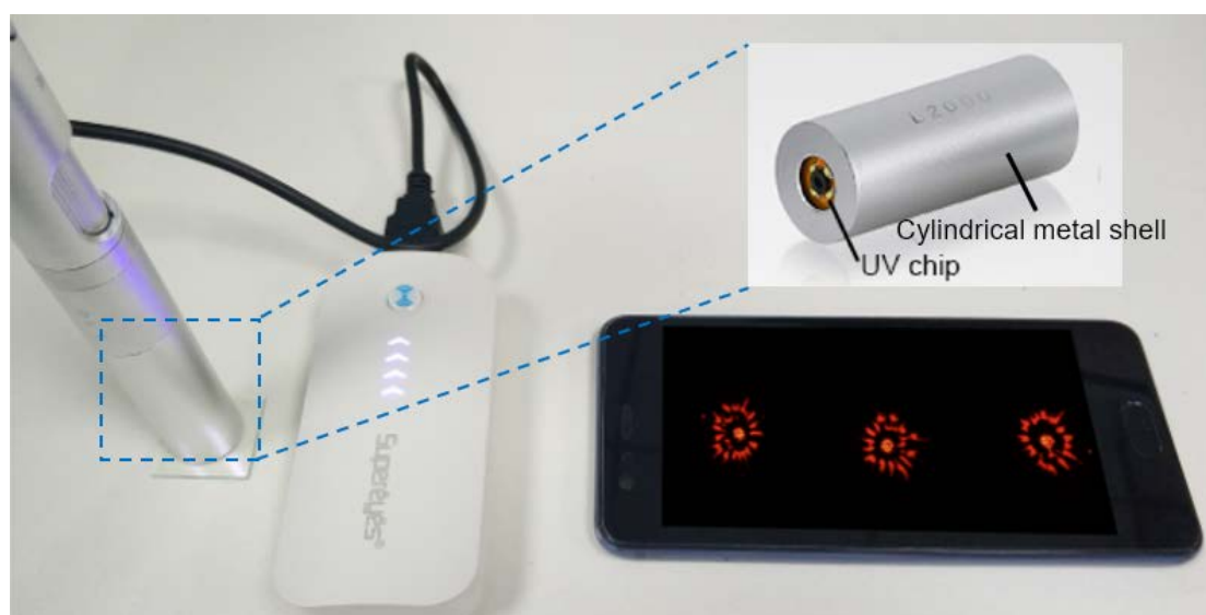
Figure S7 Pattern readout with a smartphone microscope: the portable mini-microscope is composed of a UV chip, a 200 \times magnification-adjustable objective lens covered with a cylindrical metal shell and a small WiFi box. The insert is an enlarged view of the light source and the lens.
