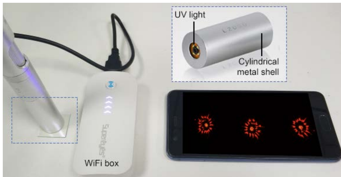
Figure S7 Pattern readout with a smartphone microscope: the portable mini-microscope is composed of a UV chip, a 200× magnification-adjustable objective lens covered with a cylindrical metal shell and a small WiFi box. The insert is an enlarged view of the light source and the lens.
