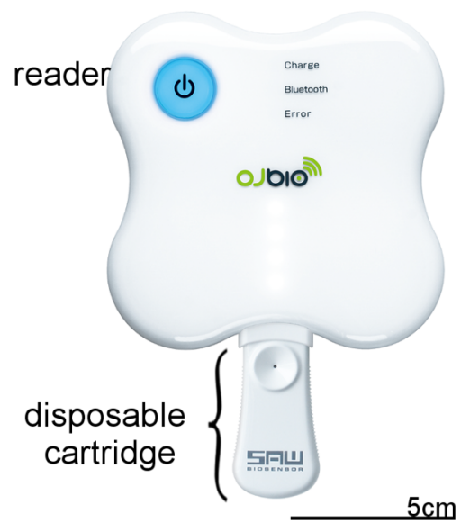
Supplementary Figure 5. Prototype SH-SAW biosensor comprising a reader with inserted disposable cartridge (including biochip), controlled by a smartphone app. The disposable cartridge-enclosed biochip limits contaminants.
