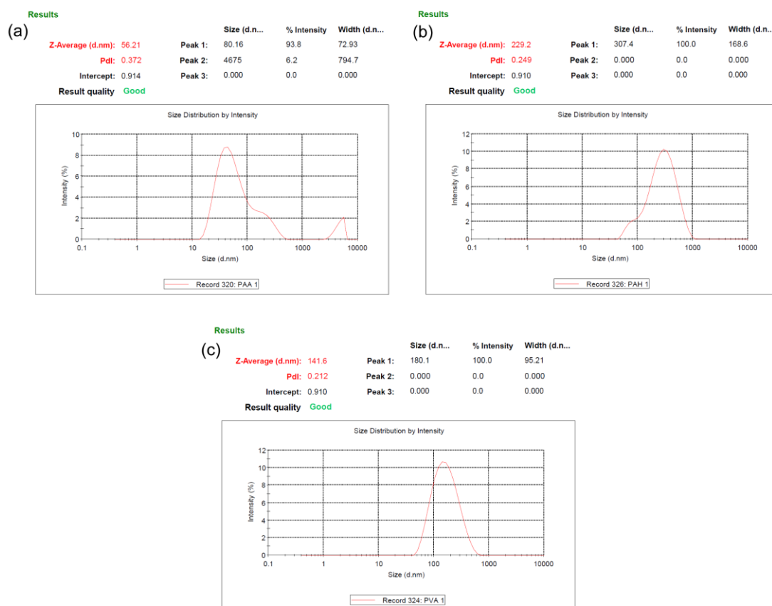
Figure S2. The hydrodynamic size profile of (a) \text{Fe}_3\text{O}_4 -PAA, (b) \text{Fe}_3\text{O}_4 -PAH and (c) \text{Fe}_3\text{O}_4 -PVA nanoparticles in aqueous suspension.
