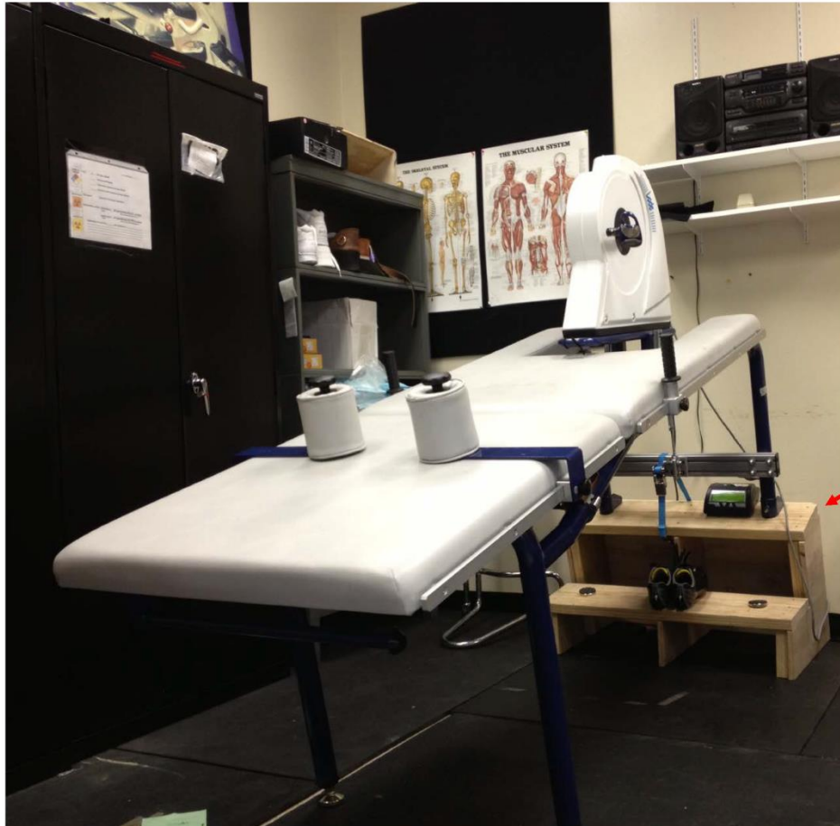
eFigure 1. Cycle ergometer modifications to achieve -15^\circ head-down tilt to induce a cephalad-fluid shift that is analogous to microgravity conditions during spaceflight.
