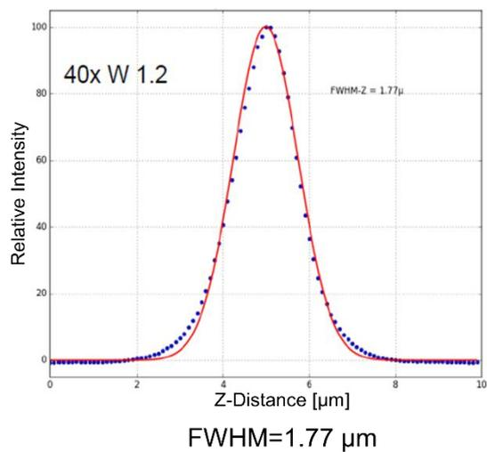
**Figure S6.** A typical confocality calibration curve of the FLUMIAS-TEXUS microscope system. The fluorescence signal of a thin layer is plotted as a function of the objective lens' z-position. The fluorescing thin layer was excited with 488nm and the signal was recorded with a sCMOS camera. The blue dots represent single measurement points with a 100nm step size. The red curve represents the mathematical interpolation.
