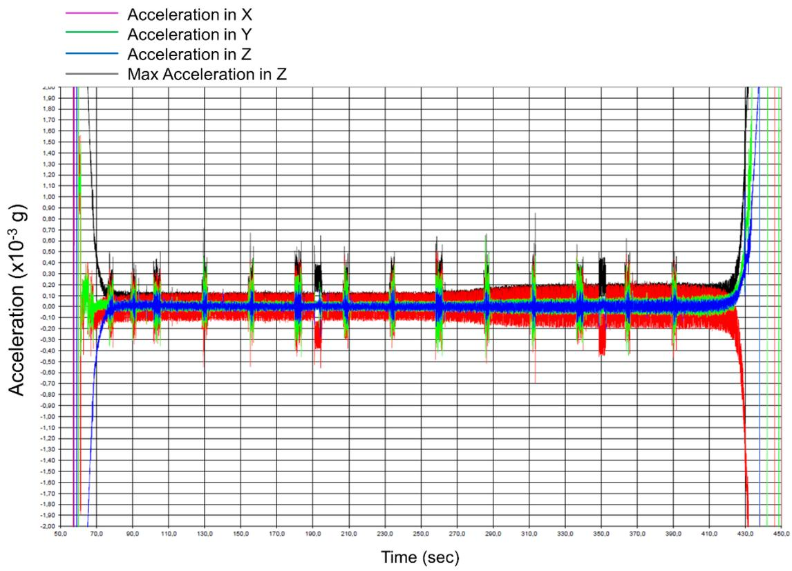
**Figure S1.** Gravity profile of the TEXUS-54 flight. Recording provided by OHB System AG.
