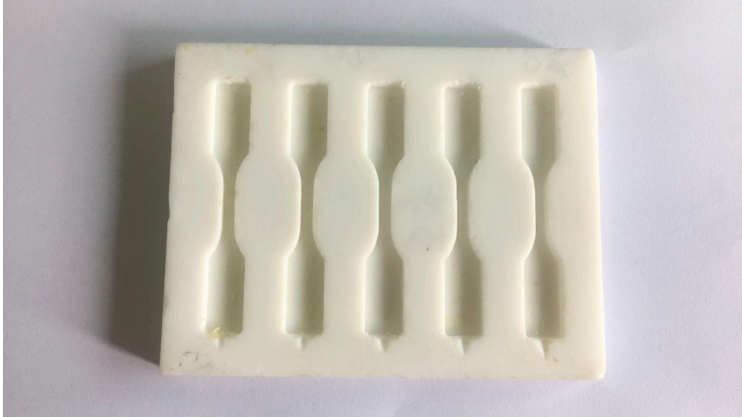
Fig. S2 PTFE mold used for preparing samples of tensile property test (Shape: Dumbbell; Length overall: 63.5 mm; Width overall: 9.53 mm; Size of the narrow middle part: 9.53 \times 3.18 \times 3.2 \text{ mm}^3 )
