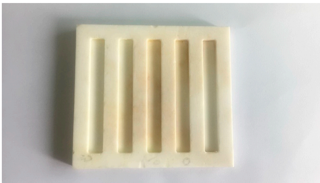
Fig. S1 PTFE mold used for preparing samples of DMA test (Shape: Cuboid; Size: 80×10×4 mm 3 )
