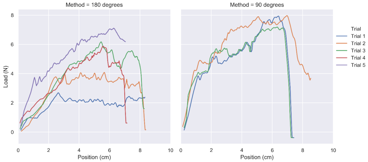
Figure S15: 90-degree and 180-degree bond strength test results; each series is a new patch (all 5 cm × 7 cm). The results of the peel test for three samples (each a different color) are plotted in the Figure S15 and show load variation due to variability of the skin (e.g., elasticity, hair density); nevertheless, the data reveal a bond strength in the range of 2–8 N for a peel distance of 5 cm (equivalent to 103–412 g/in), a range comparable to that of commercial bandages. [2]
