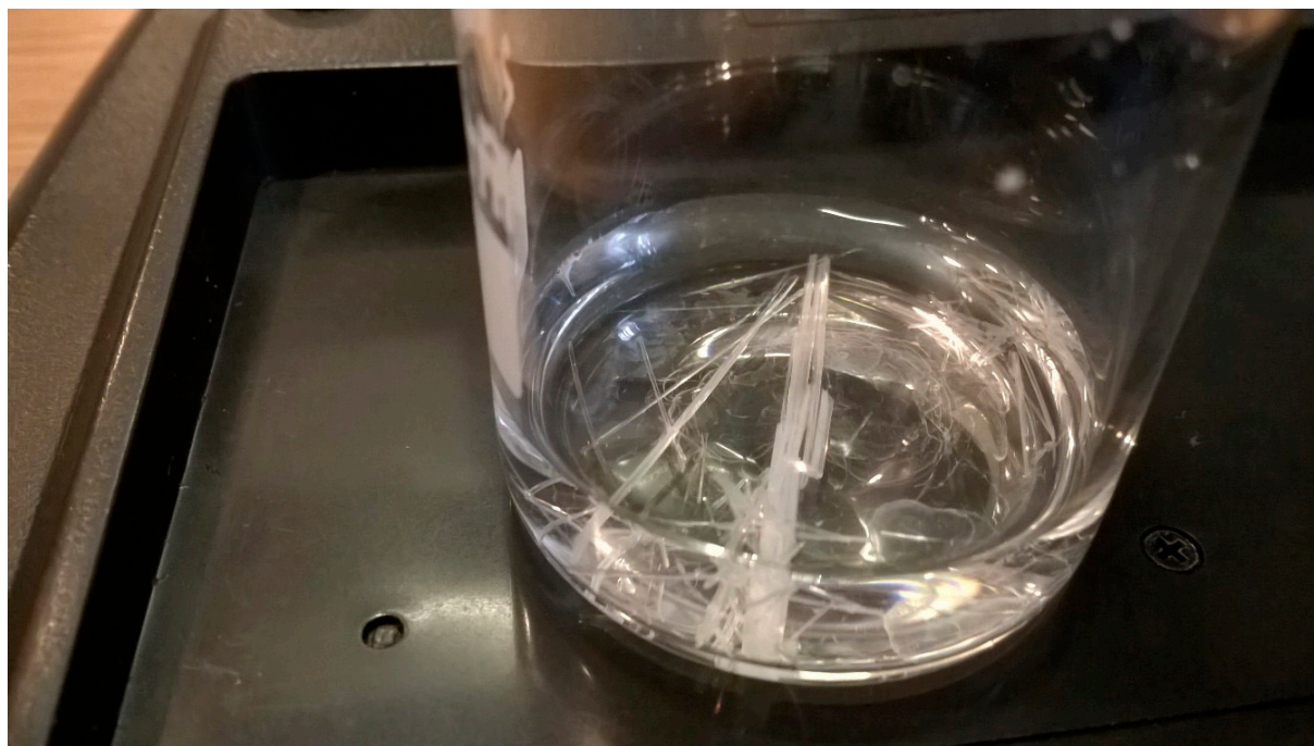
Figure S1. Photograph of silver(I) complex of metronidazole obtained as a result of one-step synthesis.
