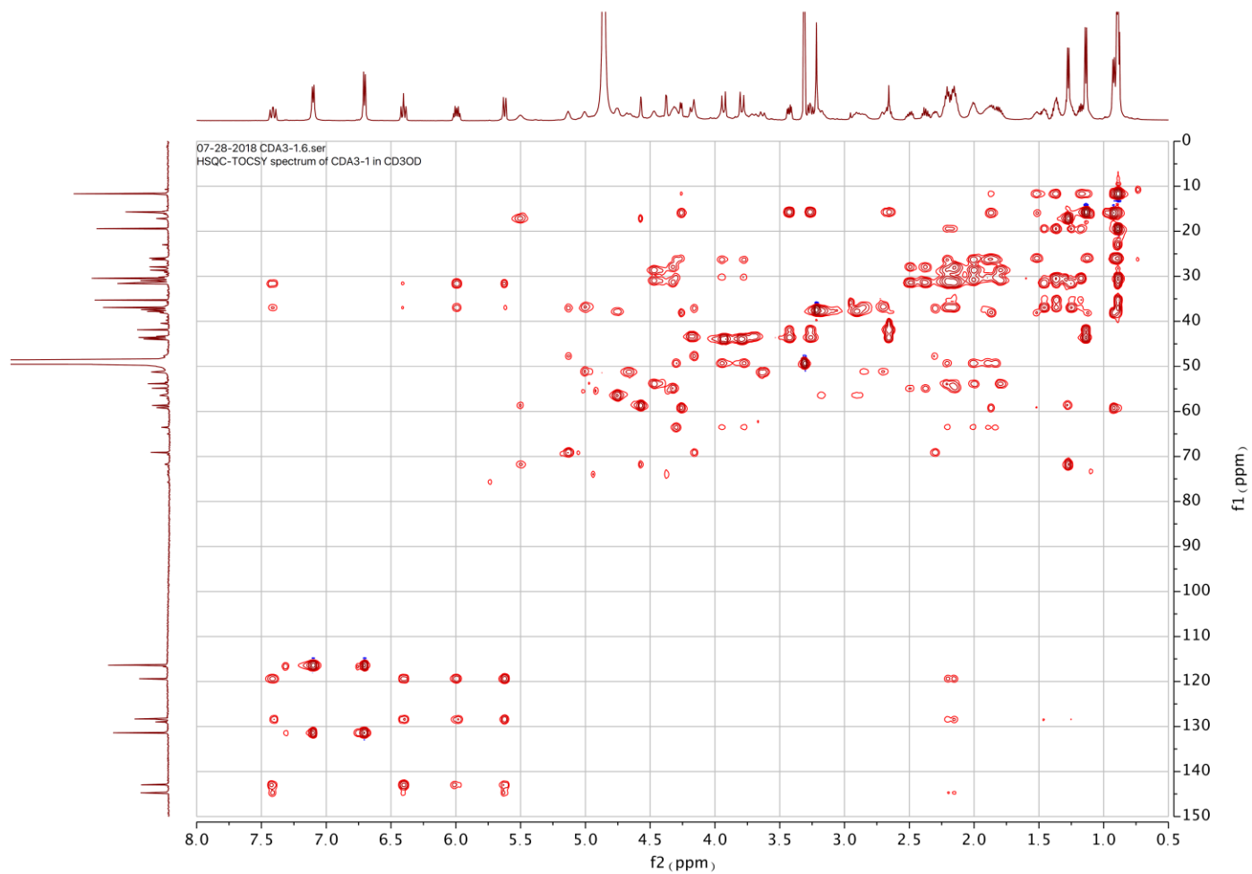
Figure S20. ^1\text{H} - ^{13}\text{C} HSQC-TOCSY NMR (600 MHz, \text{CD}_3\text{OD} ) spectrum of cadaside A ( 1 )
