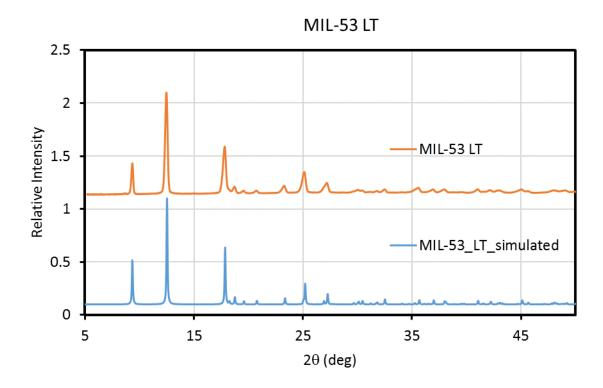
Figure S1. Powder X-Ray diffraction pattern for MIL-53 LT and its simulated pattern.
