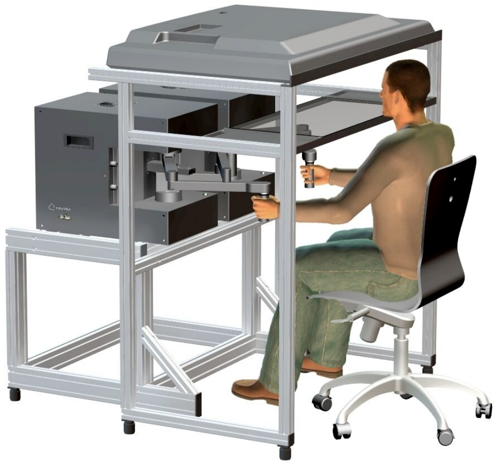
Figure 2. Three-dimensional animated representation of the KINARM End-Point robotic set-up used at 3- and 12-month follow up assessments.
