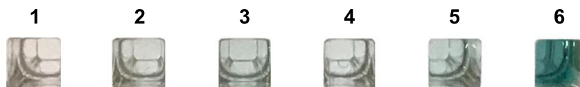
Figure S16. Utilizing MDPV-CBSAzyme for the naked-eye detection of MDPV. Experimental setup shows sample contents and photographs depict the color of the samples containing (1) reaction buffer alone, (2) 1 \mu\text{M} hemin alone, (3) 1 \mu\text{M} short fragment with hemin, (4) 1 \mu\text{M} long fragment with hemin, and both fragments in the (5) absence and (6) presence of 250 \mu\text{M} MDPV after 15 minutes of reaction.
