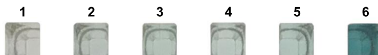
Figure S9. Utilizing COC-CBSAzyme for the naked-eye detection of cocaine. Experimental setup shows sample contents and photographs depict the color of the samples containing (1) reaction buffer alone, (2) 1 \mu\text{M} hemin alone, (3) 1 \mu\text{M} short fragment with hemin, (4) 1 \mu\text{M} long fragment with hemin, and both fragments in the (5) absence and (6) presence of 250 \mu\text{M} cocaine after 15 minutes of reaction.
