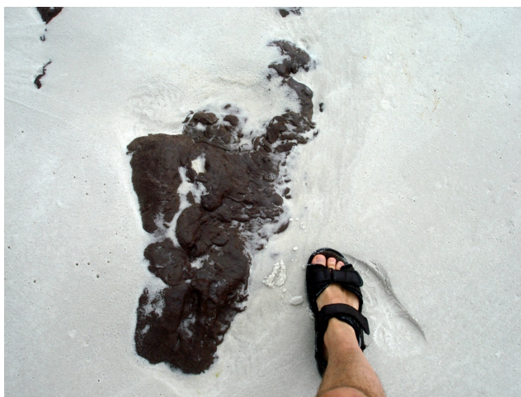
Figure S7. Partly exposed large SOA buried in Pensacola Beach sands after the Deepwater Horizon accident. This SOA was approximately 82 cm long, 42 cm wide and 25 cm thick, with a volume of 87700 cm 3 , or 2500 times larger than our experimental sSOAs (Photo Huettel, 30 th June 2010)
