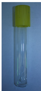
Home-made baffled culture tube for in vivo P450 BM3 activity assays, allowing for thorough aeration (required for P450 activity) while minimizing the total culture volume (and hence the quantity of 1b ). Accommodates ~3mL of culture.
