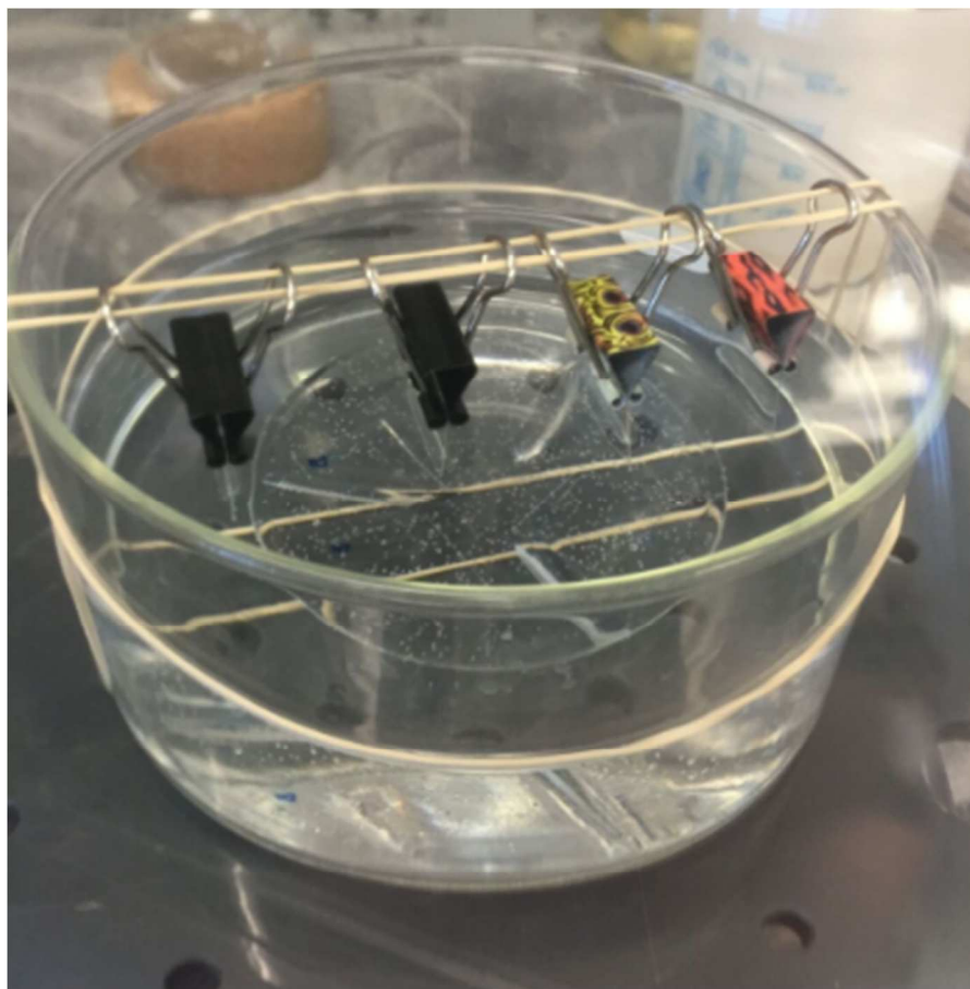
Figure S3. Apparatus used for the preparation of slides half coated with polymer 6 and half with polymer 7 . Glass cover slips were first spin coated with linear polymer 5 , then incubated in a 180 °C oven under vacuum overnight to provide crosslinked polymer 6 . The slides were then supported by clips and partially immersed in a solution of methanolic NaOH to facilitate (partial) hydrolysis of surface ester groups.
