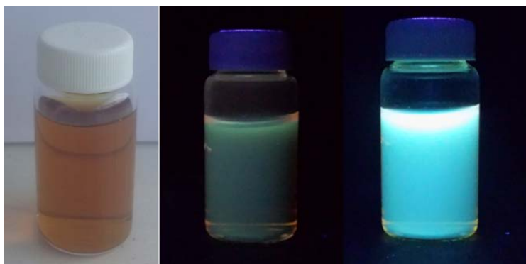
Figure S8. Images of an aqueous dispersion of C-dots with room lights on (left), room lights off but UV illumination on at 254 nm (center) and 365 nm (right).
