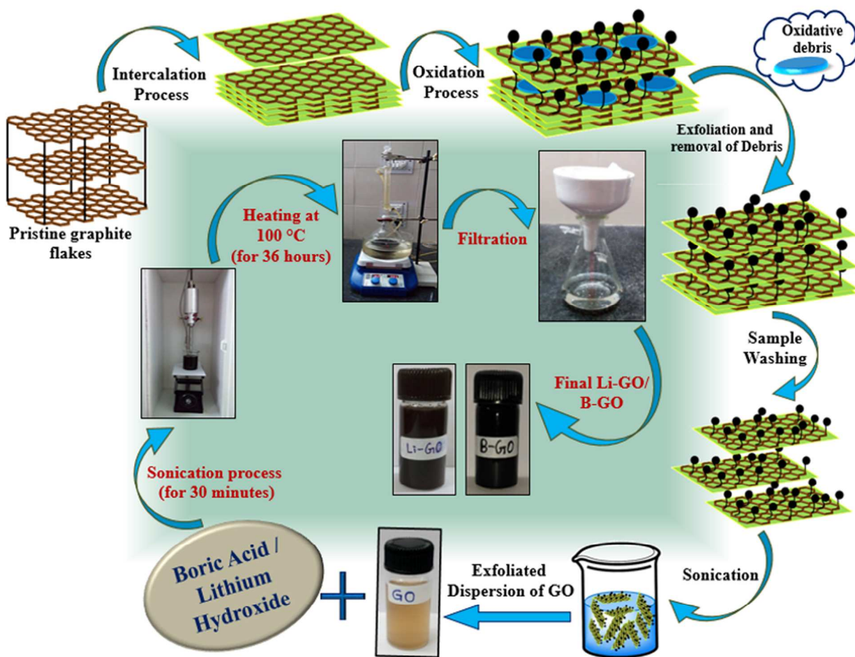
Figure S1. Schematic synthesis process of undoped GO, Li-doped GO and B-doped GO
