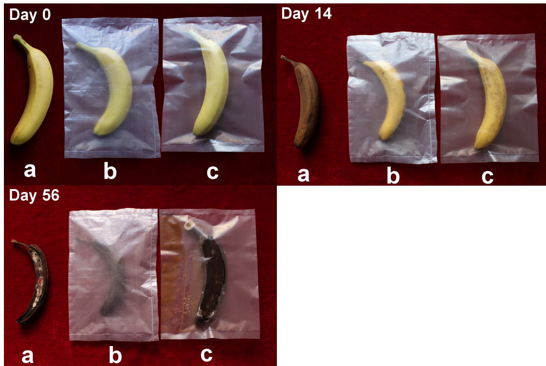
Figure S2. Photographs of banana samples with following treatment: (a) exposed to air, (b) packaged with OLDH-1 film and (c) packaged with commercial polyethylene film.
