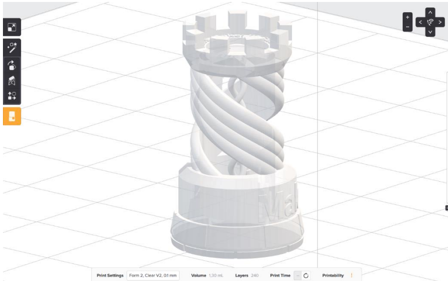
Figure S3. Graphic representation of complex shaped prototype with rook tower design, including internal helix structure, modified in PreForm software.
