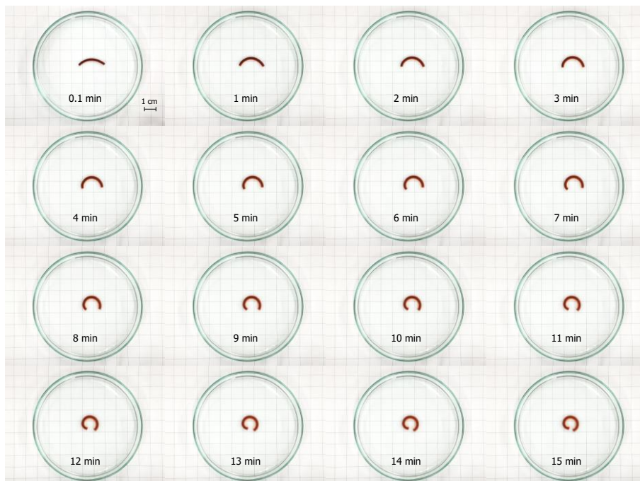
Figure S5. Time-lapsed photographs of the bending of the hydrogel bilayer (length, 2.8 cm; width, 0.3 cm; thickness, 2 mm) in a pH 7 buffer solution at 25 °C, taken every minute. The bilayer was curled into a round within 15 min.
