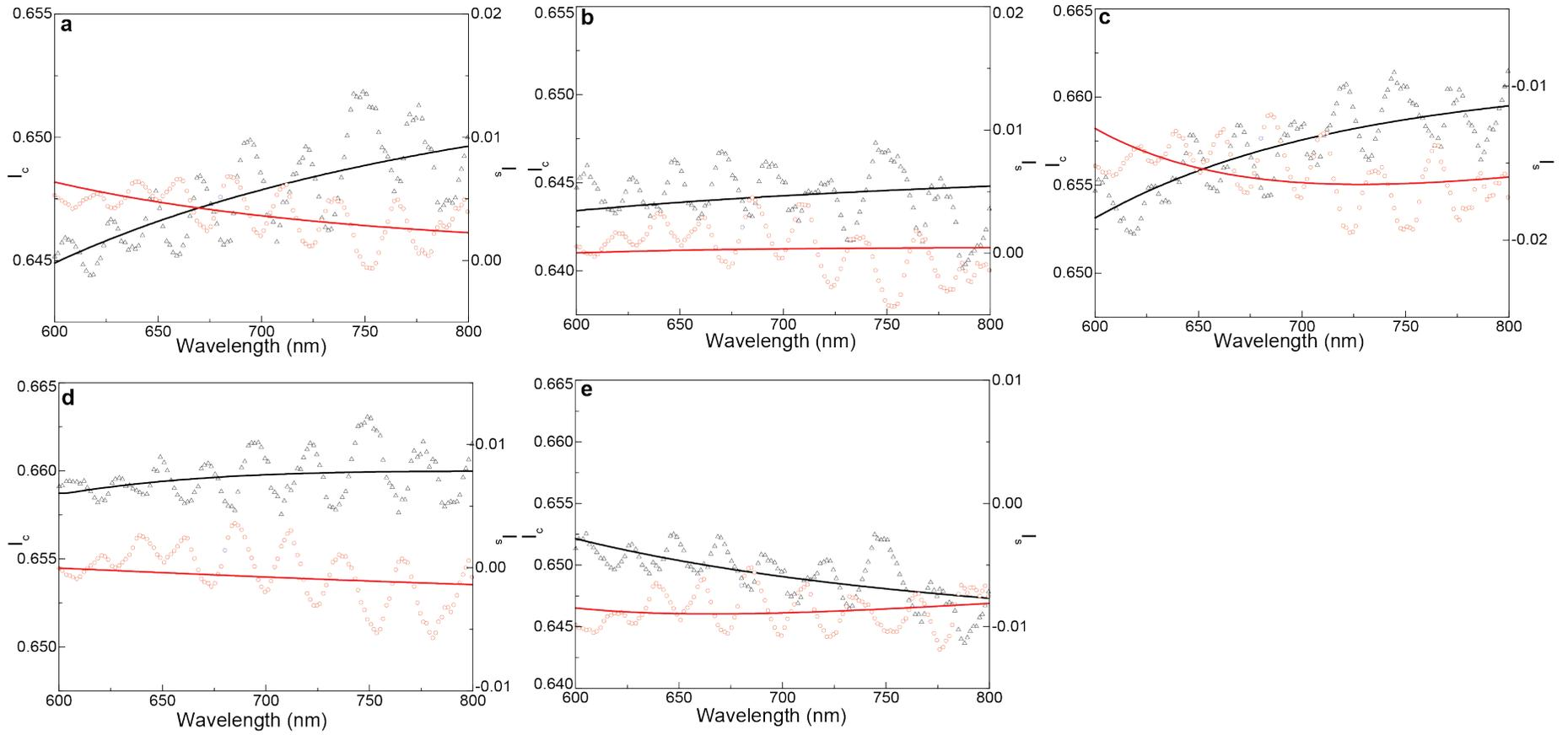
**Figure S2.** Ellipsometric parameters  $I_s$  (open circles) and  $I_c$  (open triangles) measured in PBS1-M in the regions exposed to UV radiation with energy of (a) 30; (b) 60; (c) 80; (d) 100; (e) 120  $\mu\text{J}\cdot\text{pulse}^{-1}$ . The solid lines represent the data best fit.
