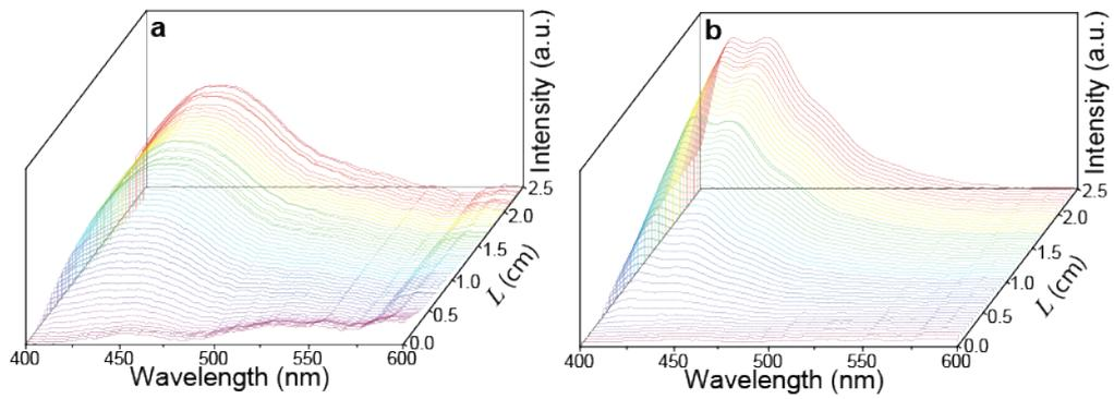
**Figure S5.** Emission spectra for different stripe lengths in (a) dU(600), (b) PBS1-M.
