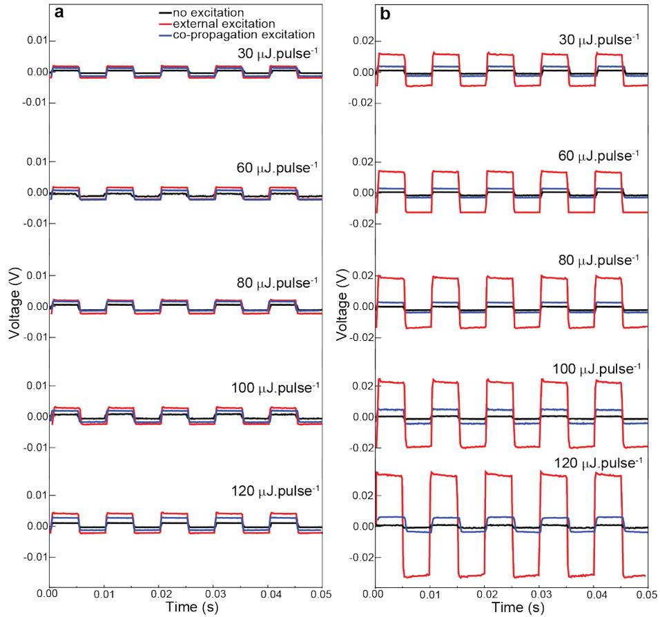
**Figure S10.** Pulsed signals at the receiver after transmission through the waveguides in (a) PBS1-M and (b) PBS2-M.
