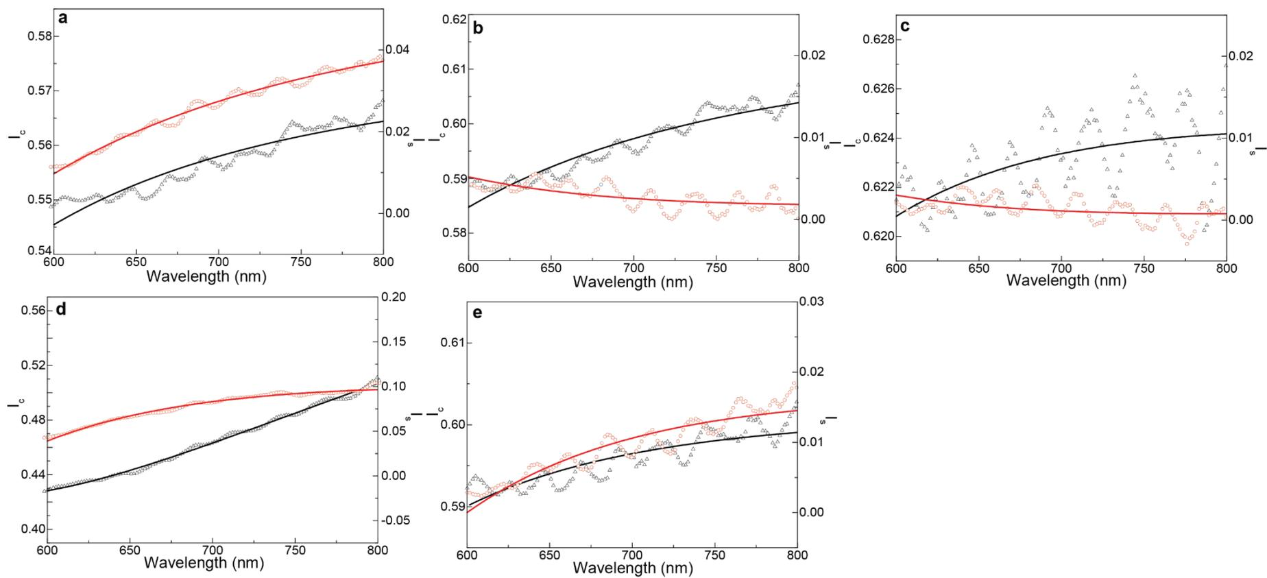
**Figure S3.** Ellipsometric parameters  $I_s$  (open circles) and  $I_c$  (open triangles) measured in PBS2-M in the regions exposed to UV radiation with energy of (a) 30; (b) 60; (c) 80; (d) 100; (e) 120  $\mu\text{J}\cdot\text{pulse}^{-1}$ . The solid lines represent the data best fit.
