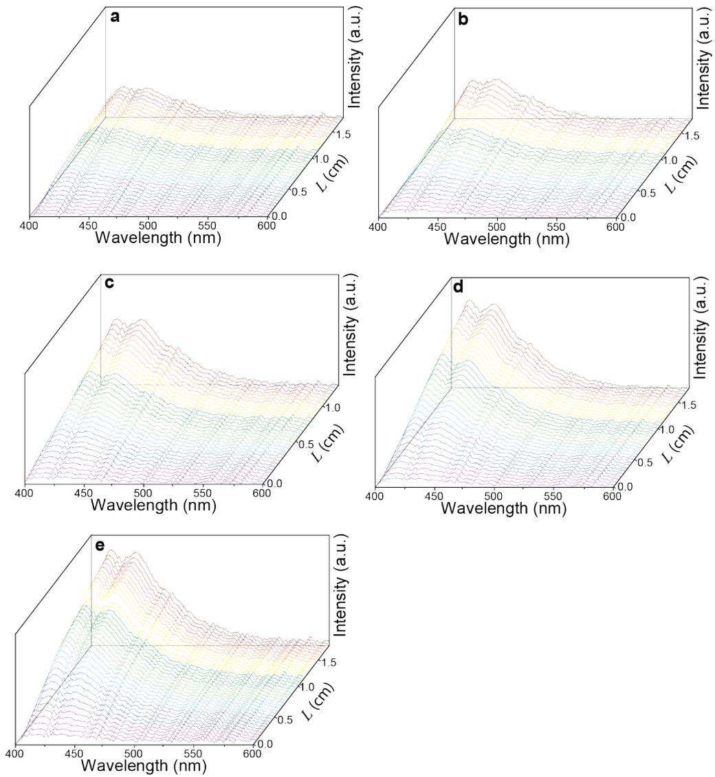
**Figure S6.** Emission spectra for different stripe lengths PBS1-M in the regions exposed to UV radiation with energy of (a) 30; (b) 60; (c) 80; (d) 100; (e) 120  $\mu\text{J}\cdot\text{pulse}^{-1}$ .
