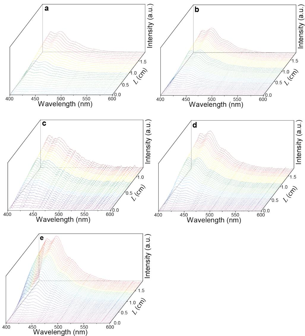
**Figure S7.** Emission spectra for different stripe lengths PBS2-M in the regions exposed to UV radiation with energy of (a) 30; (b) 60; (c) 80; (d) 100; (e) 120  $\mu\text{J}\cdot\text{pulse}^{-1}$ .
