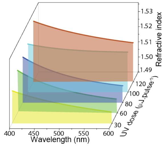
**Figure S4.** Dispersion curves obtained for the channel waveguide regions in PBS1-M.
