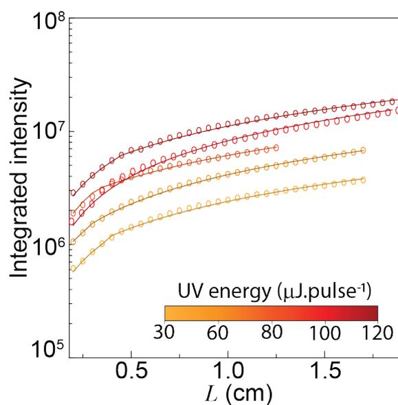
**Figure S8.** Integrated emission intensity as function of the stripe length of UV exposed regions in PBS1-M.
