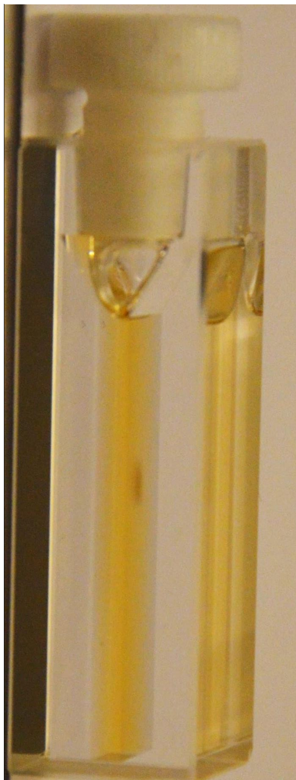
Figure S3. Pictures of a solution of \text{H}_2\text{PtCl}_6 in alkaline ethylene glycol in a 1 mm path length quartz cuvette after exposure to a UV laser. The picture is taken at an angle to see the brown spot corresponding to the formation of Pt nanoparticles.
