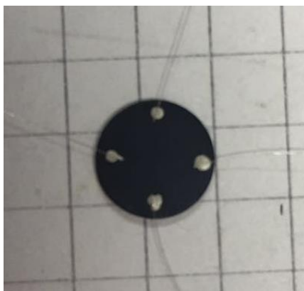
Supplementary Figure 18 | Pressed pellets device of K_3Fe_2[PcFe-O_8] for variable-temperature conductivity measurements by van der Pauw method. The powder MOF samples were pressed into pellets at 398 K under vacuum by adding \sim 1 GPa pressure. The thickness of the pressed pellet was measured as \sim 0.592 mm.
