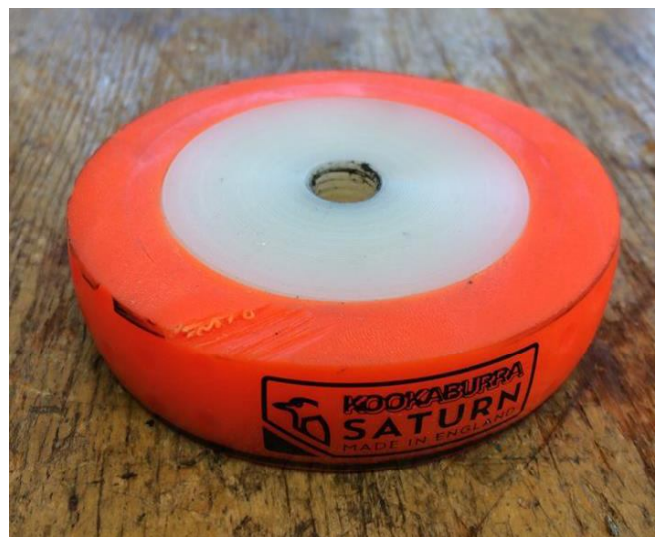
Figure S1 - Hockey ball slice impactor used in the pendulum test rig.
